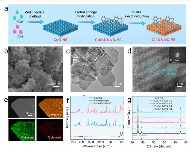
Fig. 1 Synthesis and characterization of CuO-NS-x% PS catalysts (x = 0, 10, 20, 30 and 50). (a) Schematic illustration of the synthetic procedure of Cu-NS-PS catalysts. (b) SEM, (c) TEM and (d) HRTEM images of CuO-NS-20% PS. (e) EDX elemental mappings of Cu, O and N in a single nanosheet of CuO-NS-20% PS. (f) FT-IR spectra of pure CuO-NS, proton sponge and CuO-NS-20% PS. (g) PXRD patterns of CuO-NS and CuO-NS-x% PS with different proton sponge loadings.
