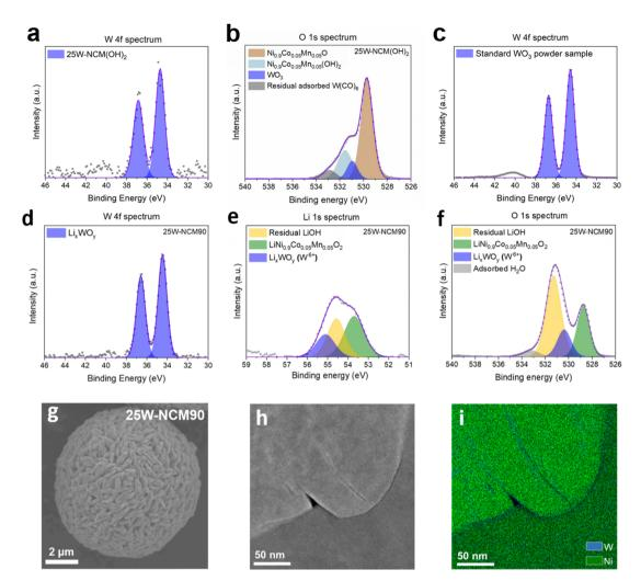
Fig. 3 XPS spectra and TEM-EDS images identifying the distribution of W and transformation of W containing compounds in 25W-NCM90. (a and b) W 4f and O 1s spectra for 25W-NCM(OH)<sub>2</sub>. (c) W 4f spectra for commercial WO<sub>3</sub> nano-powder. (d-f) W 4f, Li 1s and O 1s spectra for 25W-NCM90. (g) SEM image of a 25W-NCM90 secondary particle (h and i) TEM image and EDS elemental mapping of Ni and W along primary particle grain boundaries in 25W-NCM90.
