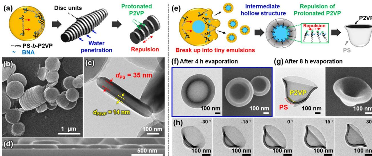
Fig. 2 (a) Schematics illustrating the proposed mechanism of the formation of disc-like particles when  $x = 1.2$ . (b–d) Representative (b) top-view SEM, (c) TEM, and (d) side-view SEM images of disc-like particles. (e) Schematics illustrating the proposed mechanism of the formation of Janus cups when  $x = 1.5$ . (f and g) TEM and SEM images of particles captured after evaporation for 4 h and 8 h, respectively. (h) TEM images of Janus cups tilted at angles of  $-30$  to  $30^\circ$ .
