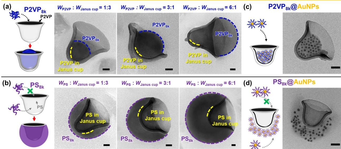
Fig. 5 Selective loading of homopolymers (hPS or hP2VP) and polymer-grafted gold NPs into PS-*b*-P2VP Janus cups. (a and b) TEM images of Janus cups loaded with different weight ratios of (a) P2VP<sub>8k</sub> and (b) PS<sub>8k</sub> homopolymers. (c and d) TEM images of Janus cups loaded with (c) P2VP<sub>8k</sub>@AuNPs and (d) PS<sub>8k</sub>@AuNPs. Scale bars are 50 nm.
