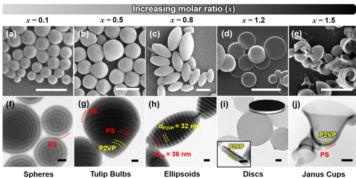
Fig. 1 SEM and TEM images of PS-*b*-P2VP(BNA) <sub>$x$</sub>  particles. (a–e) SEM and (f–j) TEM images of PS-*b*-P2VP(BNA) <sub>$x$</sub>  particles at different  $x$  values of (a and f) 0.1, (b and g) 0.5, (c and h) 0.8, (d and i) 1.2 and (e and j) 1.5. Scale bars in (a–e) are 1  $\mu\text{m}$  while 100 nm in (f–j). Inset in (i) is the cartoon of disc particles.
