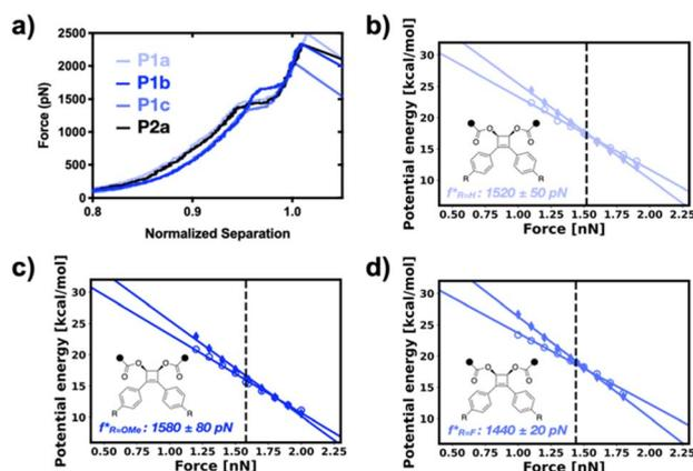
Fig. 2 (a) Representative single-molecule force spectroscopy data of cyclobutene mechanophores as a function of alkene substituent. Computed activation energies as a function of force for (b) **P1a**, (c) **P1b**, and (d) **P1c**. The conrotatory reactions are shown in open symbols; disrotatory reactions are shown in filled symbols. Vertical dashed lines correspond to the respective average plateau forces observed experimentally.
