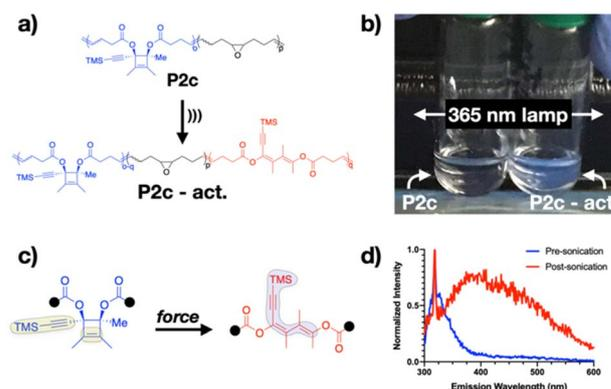
Fig. 5 (a) Sonication of **P2c** opens the cyclobutene ring, leading to observed fluorescence in the post-sonicated solution (b). The fluorescence is attributed to increased conjugation, including that into the alkyne substituent (c). (d) Emission spectrum of pre- and post-sonication solutions of **P2c**.
