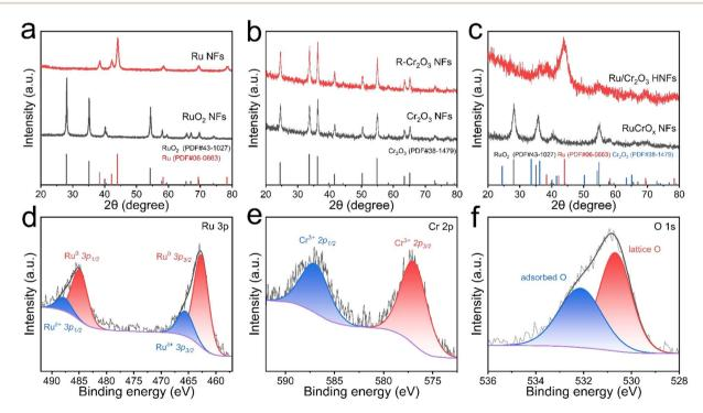
Fig. 2 XRD patterns of (a)  $RuO_2$  NFs and Ru NFs, (b)  $Cr_2O_3$  NFs and  $R-Cr_2O_3$  NFs, and (c)  $RuCrO_x$  NFs and  $Ru/Cr_2O_3$  HNFs. Typical high-resolution (d) Ru 3p, (e) Cr 2p and (f) O 1s XPS spectra of  $Ru/Cr_2O_3$  HNFs.
