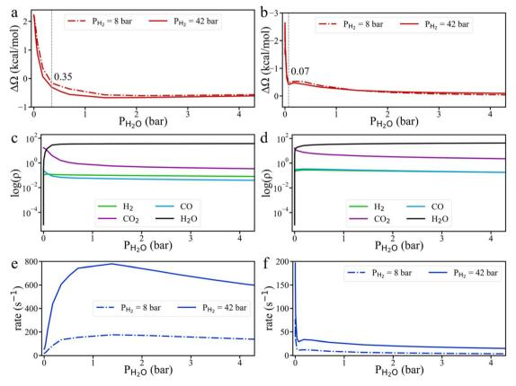
Fig. 8 The influence of  $H_2O$  partial pressure on the kinetics of  $CO_2$  hydrogenation. Variation of the grand potential barrier for HCOO\* hydrogenation on Cu (111) (a) and Cu (211) (b) surfaces. Surface gas densities on Cu (111) (c) and Cu (211) (d) under 42 bar  $H_2$  pressure. HCOO\* hydrogenation rates on Cu (111) (e) and Cu (211) (f) surfaces. All simulations were conducted at 503 K, with a fixed gas ratio of  $H_2$ :  $CO_2$ : CO = 6: 1:1.
