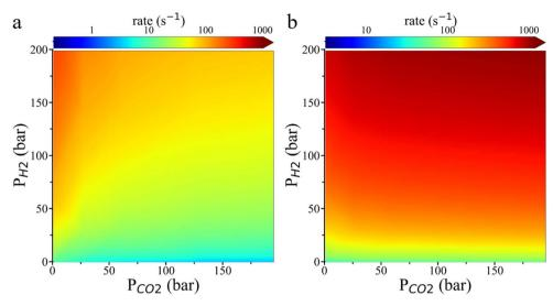
Fig. 6 Contour plot of the HCOO\* hydrogenation rate as a function of  $CO_2$  and  $H_2$  partial pressures on Cu (111) (a) and Cu (211) (b) surfaces. The reaction rate was predicted by the transition state theory with grand potential simulation at 503 K.
