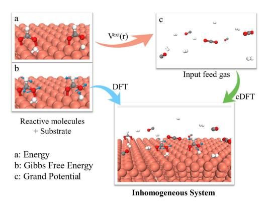
Fig. 1 Scheme of the grand potential approach to predict environmental effects on heterogeneous catalysis. (a) Calculation of substrate energy (E) with electronic DFT. (b) Free energy correction to account for the bond vibrational entropy, which is referred to as the Gibbs free energy in this work. (c) Calculation of the grand potential ( $\Omega$ ) of the entire inhomogeneous system with cDFT.
