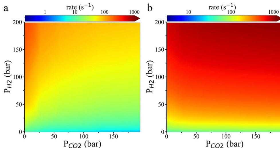
Fig. 6 Contour plot of the HCOO\* hydrogenation rate as a function of CO<sub>2</sub> and H<sub>2</sub> partial pressures on Cu (111) (a) and Cu (211) (b) surfaces. The reaction rate was predicted by the transition state theory with grand potential simulation at 503 K.
