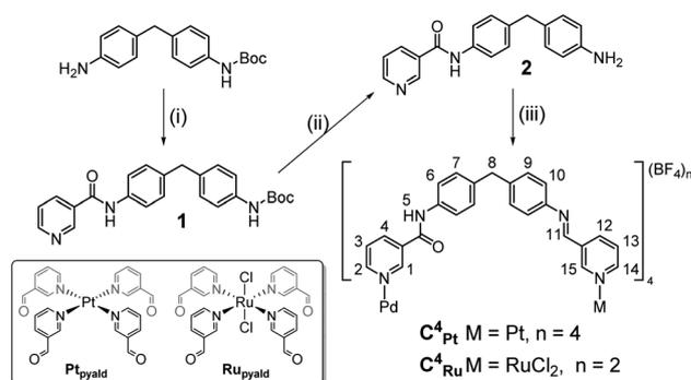
Scheme 1 Synthetic route to low-symmetry  $\text{PdPt C}^4_{\text{Pt}}$  and  $\text{PdRu C}^4_{\text{Ru}}$  cages. Reaction conditions: (i) nicotinic acid, HATU, TEA,  $\text{CH}_3\text{CN}$ , reflux, 16 h. (ii) TFA :  $\text{CHCl}_3$  (1 : 5), 3 h. (iii)  $[\text{Pd}(\text{CH}_3\text{CN})_4](\text{BF}_4)_2$ ,  $\text{Pt}_{\text{pyald}}$  or  $\text{Ru}_{\text{pyald}}$ , DMSO, 24 h.
