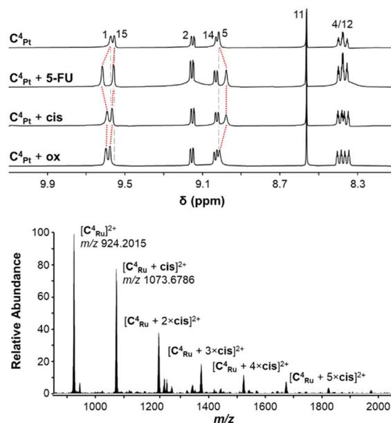
Fig. 8 (top) <sup>1</sup>H NMR spectra (CD<sub>3</sub>CN, 298 K, 400 MHz) of  $C^4_{Pt}$  and mixtures of  $C^4_{Pt}$  with 5-FU, *cis*, or *ox* (1 : 5). Shifts of *endo*-facing protons H-1, H-5, and H-15 are shown with dashed red lines. Vertical grey lines indicate the same chemical shift for the corresponding peak of  $C^4_{Pt}$  (top spectrum). (bottom) ESI-mass spectrum of a 1 : 5 mixture of  $C^4_{Ru}$  and *cis*.
