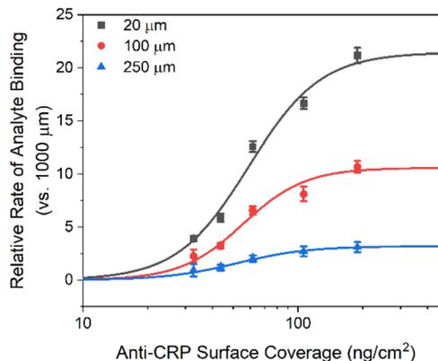
Fig. 6 The impact of microfluidic flux enhancement as a function of (SPR determined) antibody surface density. The binding rate was normalized as the ratio of the temporal  $C_r$  change in response to 10  $\mu\text{g mL}^{-1}$  CRP samples within microfluidic channels of 20, 100, and 250  $\mu\text{m}$  versus 1000  $\mu\text{m}$  height, respectively. Error bars represent the standard deviation across three individual electrodes ( $n = 3$ ).
