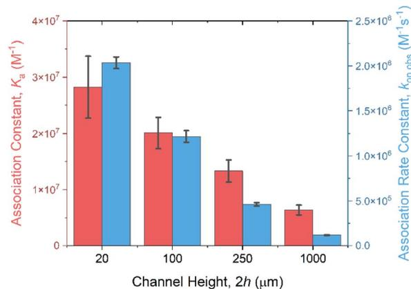
Fig. 5 The effect of microfluidic channel height  $2h$  on the association constant  $K_a$  (red) and the observed association rate constant  $k_{on,obs}$  (blue).  $K_a$  was determined using the Langmuir–Freundlich isotherms model by fitting equilibrium data of the capacitive response ( $C_r$  in plateau) versus analyte concentration (Fig. S16†).  $k_{on,obs}$  was derived from the first-order kinetic fitting of association  $C_r$  response, as detailed in Experimental section, ESI†.
