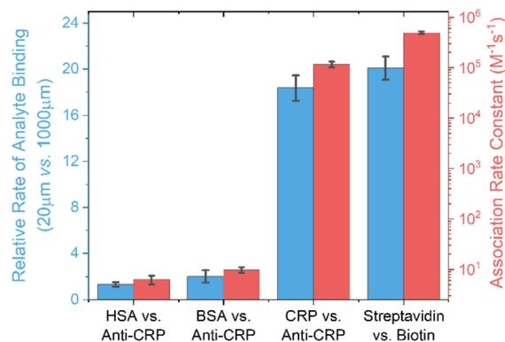
Fig. 7 The strong resolved correlation between the enhancement of target binding rate on channel compression and the association rate constant  $k_{on}$  for nonspecific (HSA/anti-CRP, BSA/anti-CRP) and specific (CRP/anti-CRP, streptavidin/biotin) biorecognition pairs. Association rate constants were derived from SPR sensograms, as detailed in the Experimental section, ESI†.
