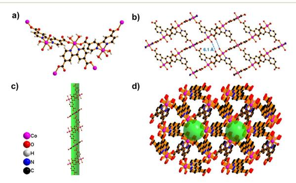
Fig. 1 (a) Coordination environment. (b) View of interpenetrated 2D sheets along the *b*-axis. (c) 1D channels along the *c*-axis. (d) View showing the decorated cages in the 3D framework. Hydrogen atoms are omitted for clarification.
