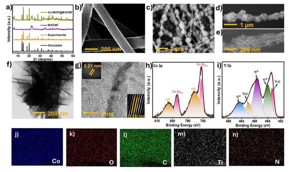
Fig. 2 Characterization of Co-MOF@MXCNF. (a) PXRD patterns. FESEM images of (b) MXCNF and (c-e) Co-MOF@MXCNF at high and low magnification. (f) TEM image of Co-MOF@MXCNF. (g) HRTEM images of Co-MOF@MXCNF (inset: IFFT image). XPS high-resolution spectra of (h) Co 2p and (i) Ti 2p. EDS mapping of Co-MOF@MXCNF: (j) cobalt (Co), (k) oxygen (O), (l) carbon (C) (red), (m) titanium (Ti), and (n) nitrogen (N) elements.
