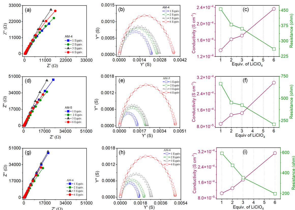
Fig. 6 Nyquist plots of SONs doped with varying equivalents of  $\text{LiClO}_4$  for (a) AM-4, (d) AM-5, and (g) AM-6, respectively. Corresponding admittance plots for SONs of (b) AM-4, (e) AM-5, and (h) AM-6, respectively. Corresponding plot of resistance and conductivity data with varying equivalents of  $\text{LiClO}_4$  for SONs of (c) AM-4, (f) AM-5, and (i) AM-6, respectively.
