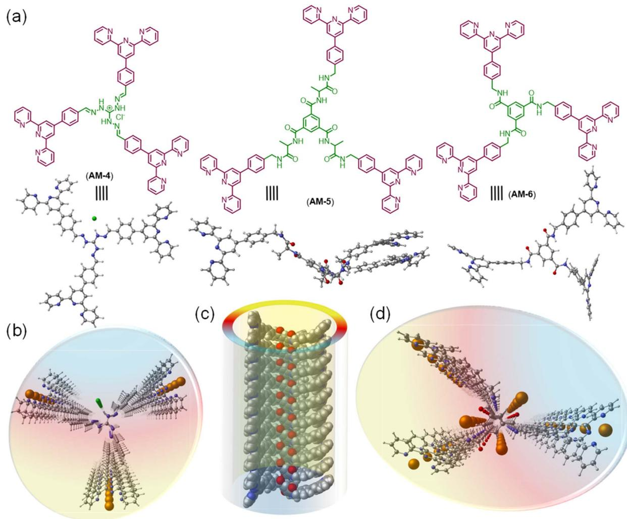
**Fig. 1** (a) Chemical and computationally optimized structures of  $C_3$ -symmetrical molecules AM-4, AM-5, and AM-6, respectively. (b) Schematic representation of the top view of the SONs of AM-4 with Li-ion migration. (c and d) Schematic representation of the SONs of AM-6 with Li-ion migration through possible binding pockets (carbon = grey; nitrogen = blue; oxygen = red; chloride = green; Li = orange).
