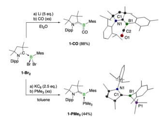
Fig. 1 Synthesis of the CO (1-CO) and PMe<sub>3</sub> (1-PMe<sub>3</sub>) adducts of CAAC-bound mesitylborylene. Molecular structures are shown with thermal ellipsoids at 50% probability. The thermal ellipsoids for the aryl and alkyl substituents, along with hydrogen atoms, are omitted. Selected bond lengths (Å) and angles (°): 1-CO: C2-O11.163(2), B1-C11.500(2), B1-C21.466(2), N1-C11.358(2); O1-C2-B1171.3(1); 1-PMe<sub>3</sub>: B1-P11.934(1), B1-C11.462(2), N1-C11.433(1); C1-B1-P1124.14(9).
