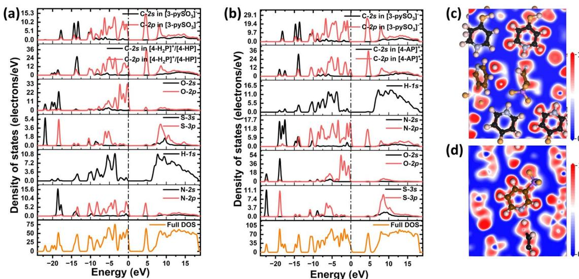
Fig. 3 Calculated density of states of (a) compound 1 and (b) compound 2; calculated ELF diagrams of (c) [4-H<sub>2</sub>P]<sup>+</sup>/[4-HP] and (d) [3-pySO<sub>3</sub>]<sup>-</sup> groups in compound 1.
