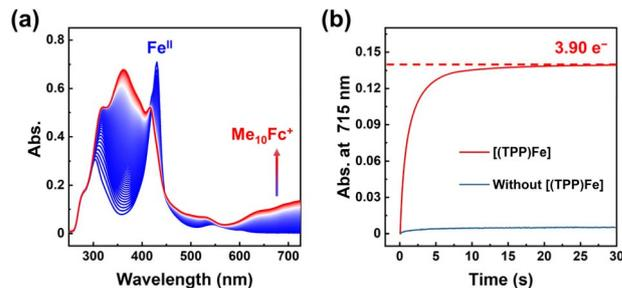
Fig. 3 (a) UV-vis spectra observed during the chemical ORR with  $[(\text{TPP})\text{Fe}^{\text{III}}]\text{ClO}_4$ . (b) Time profiles of the  $\text{Me}_{10}\text{Fc}^+$  formation during the chemical ORR with and without  $[(\text{TPP})\text{Fe}^{\text{III}}]\text{ClO}_4$ .
