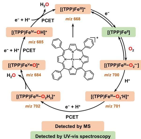
Scheme 2 Proposed mechanism of the  $4\text{e}^-/4\text{H}^+$  ORR with  $[(\text{TPP})\text{Fe}^{\text{III}}]^+$  as the catalyst.<sup>12,20,31,33,77</sup>
