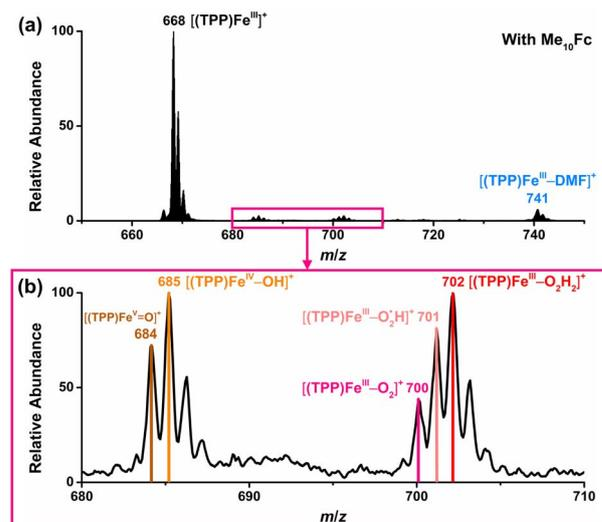
Fig. 4 Mass spectra of the chemical ORR catalyzed by  $[(\text{TPP})\text{Fe}^{\text{III}}]^+$  with  $\text{Me}_{10}\text{Fc}$  as the reductant in DMF. (a) Full-scale mass spectra. (b) Zoomed-in mass spectra of iron-oxygen intermediates.
