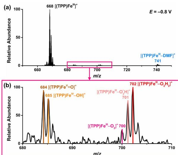
Fig. 2 Mass spectra of the electrochemical ORR catalyzed by  $[(\text{TPP})\text{Fe}^{\text{III}}]^+$  in DMF when the voltage was at  $-0.8$  V vs.  $\text{Fc}^+/\text{Fc}$ . (a) Full-scale mass spectra. (b) Zoomed-in mass spectra of iron-oxygen intermediates.
