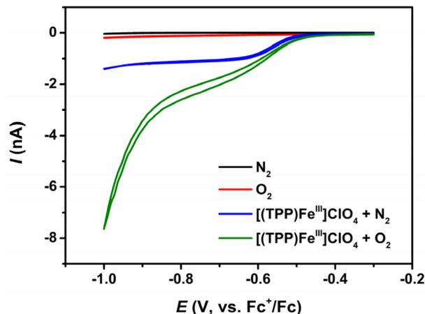
Fig. 1 CV curves of 0.5 mM  $[(\text{TPP})\text{Fe}^{\text{III}}]\text{ClO}_4$  in the absence (blue) and presence (green) of 1 atm  $\text{O}_2$  on a carbon UME in DMF (Cell 1). Black (with  $\text{N}_2$ ) and red (with  $\text{O}_2$ ) curves are the potential windows of the carbon UME using Cell 1 without  $[(\text{TPP})\text{Fe}^{\text{III}}]\text{ClO}_4$ .
