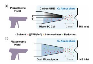
Scheme 1 Schematic illustration of the *in situ* MS setups to study (a) electrochemical and (b) chemical ORRs mediated by [(TPP)Fe<sup>III</sup>]<sup>+</sup>.
