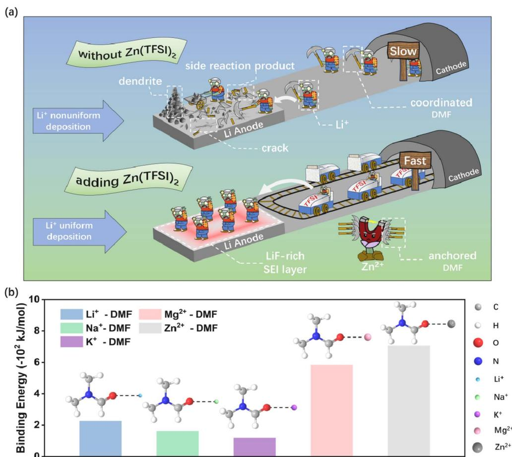
Fig. 1 (a) Schematic illustration for the action mechanism of  $\text{Zn}(\text{TFSI})_2$  in PVDF-based electrolyte. (b) The binding energy of  $\text{Li}^+$ –DMF,  $\text{Na}^+$ –DMF,  $\text{K}^+$ –DMF,  $\text{Mg}^{2+}$ –DMF and  $\text{Zn}^{2+}$ –DMF.
