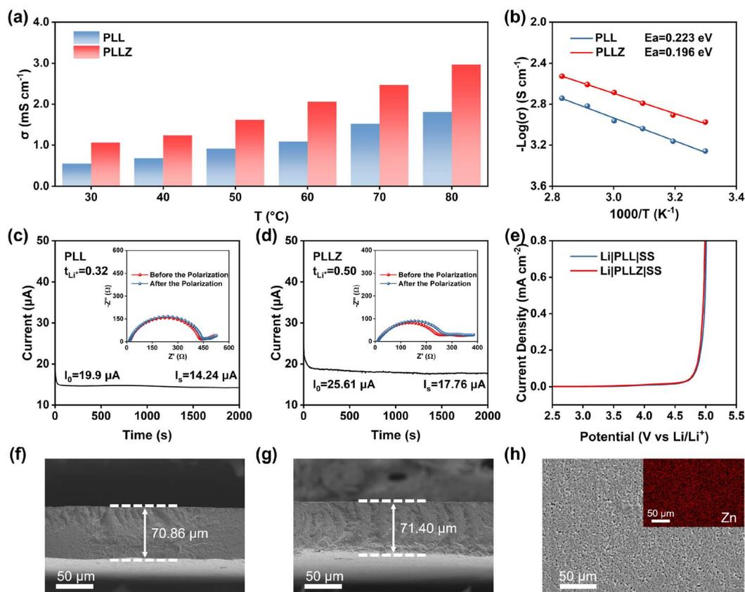
Fig. 3 (a) The ionic conductivities and (b) Arrhenius plots of PLL and PLLZ electrolytes in the temperature range from 30 to 80 °C. Chronoamperometry curves and Nyquist plots (inset) before and after the polarization of (c) Li|PLL|Li and (d) Li|PLLZ|Li symmetric cells. (e) LSV curves of PLL and PLLZ electrolytes. Cross-sectional SEM images of (f) PLL and (g) PLLZ electrolytes. (h) Surface SEM and corresponding EDS mapping images of PLLZ electrolyte.
