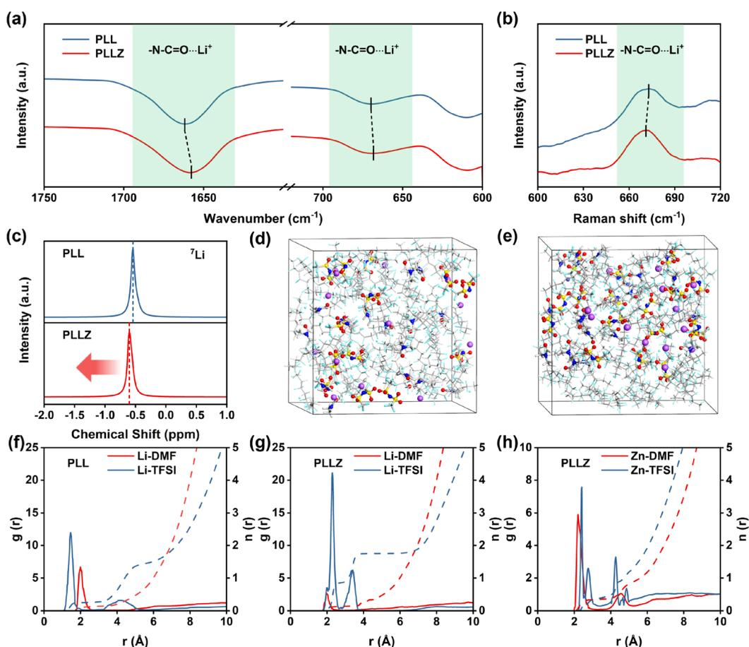
Fig. 2 (a) FTIR spectra of PLL and PLLZ electrolytes. (b) Raman spectra of PLL and PLLZ electrolytes. (c) <sup>7</sup>Li NMR spectra of PLL and PLLZ electrolytes. Snapshots of (d) PLL and (e) PLLZ electrolytes from molecular dynamics simulations. Radial distribution functions of Li<sup>+</sup>-DMF and Li<sup>+</sup>-TFSI<sup>-</sup> in (f) PLL and (g) PLLZ electrolytes. (h) Radial distribution functions of Zn<sup>2+</sup>-DMF and Zn<sup>2+</sup>-TFSI<sup>-</sup> in PLLZ electrolytes.
