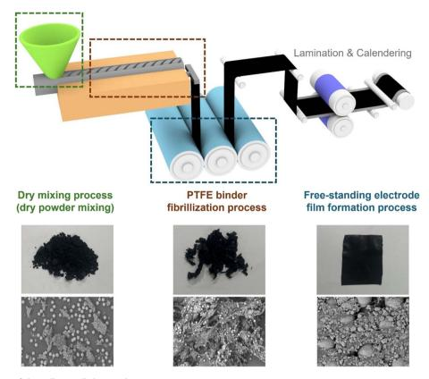
Fig. 5 Main processes of the roll-to-roll dry coating process
