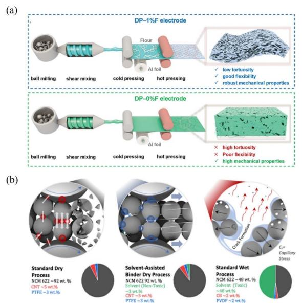
Fig. 11 Improvement of mechanical properties of dry electrodes (LIBs): (a) fabrication procedures of DP-1% F and DP-0% F electrodes. Reproduced with permission from ref. 100. Copyright (2024) Wiley-VCH GmbH. (b) Fracturing of active materials, effects of the solvent-assisted-binder (SaB) dry process, and capillary stresses in relation to mixture composition during dry processing. Reproduced with permission from ref. 101. Copyright (2023) The Authors. Published by Elsevier B.V.
