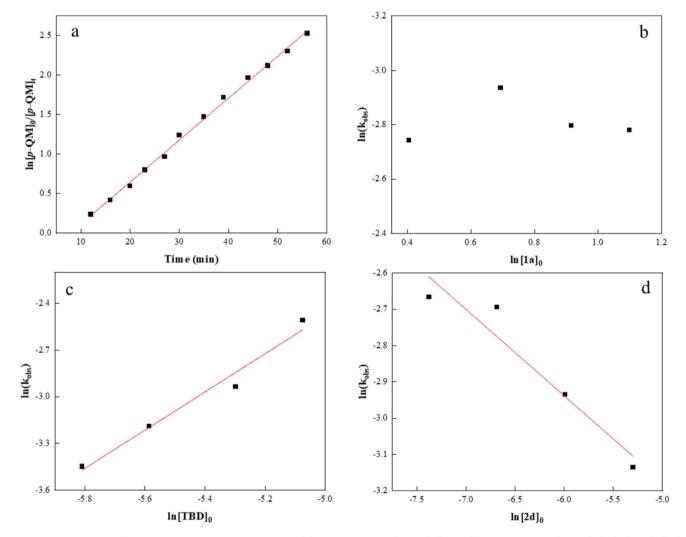
Fig. 3 Kinetics for p-QM/isothiocyanate **1a** copolymerization: (a) kinetic plot of  $\ln([p-QM]_0/[p-QM]_t)$  versus time at a  $[p-QM]_0/[1a]_0/[TBD]_0/[2d]_0$  ratio of 100: 400: 1:0.5. (b) Plot of  $k_{obs}$  versus [1a]<sub>0</sub>. (c) Plot of  $\ln(k_{obs})$  versus  $\ln[TBD]_0$ . (d) Plot of  $\ln(k_{obs})$  versus  $\ln[2d]_0$ .
