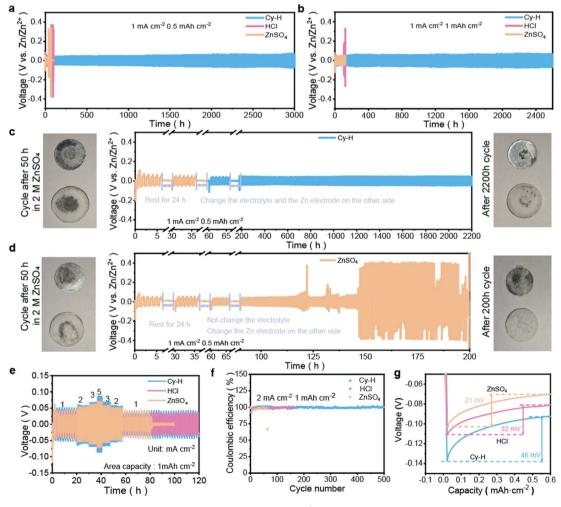
Fig. 3 Voltage profiles of  $Zn\|Zn$  symmetric cells at (a) 0.5 and (b) 1 mA h cm<sup>-2</sup>; voltage profiles of  $Zn\|Zn$  symmetric cells with Cy-H (c) and ZSO (d) for by-product elimination; (e) rate performance of  $Zn\|Zn$  cells at different current densities; (f) CE of  $Cu\|Zn$  asymmetric cells using different electrolytes; (q) nucleation overpotential of the first cycle of  $Zn\|Cu$  asymmetric cells in different electrolytes.
