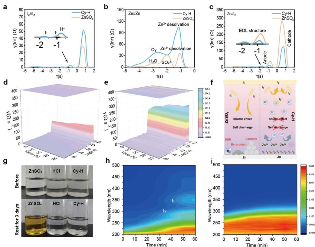
Fig. 6 DRT spectra of  $\text{I}_2||\text{I}_2$  (a),  $\text{Zn}||\text{Zn}$  (b) and  $\text{Zn}||\text{I}_2$  (c) with different electrolytes; *in situ* DRT spectra during self-discharge of Cy-H (d) and ZSO (e); schematic diagram of the self-discharge suppression mechanism (f); (g) immersion experiment in different electrolytes; *in situ* surface UV of ZSO (h) and Cy-H (i).
