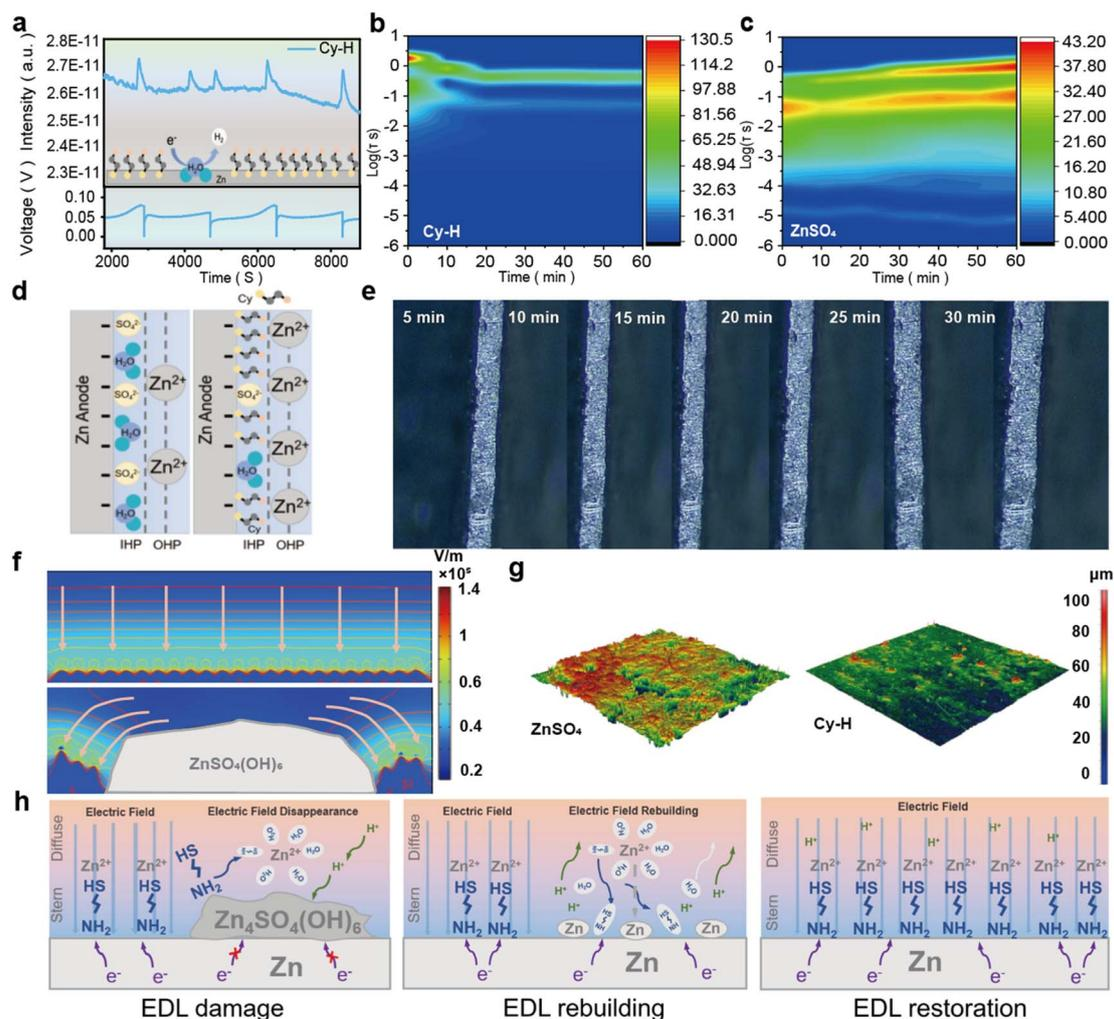
Fig. 4 (a) DEMS test pattern of Cy-H; *in situ* DRT spectra of Cy-H (b) and ZSO (c); (d) structure of EDLs with different electrolytes; (e) *in situ* optical images of the Zn plating on the Zn anode in Cy-H; (f) distribution of  $\text{Zn}^{2+}$  concentration on different electrode surfaces; (g) optical 3D surface profiler image of different electrolytes; (h) a schematic illustration of the Cy-H-specific immunological mechanism for safeguarding the Zn anode.
