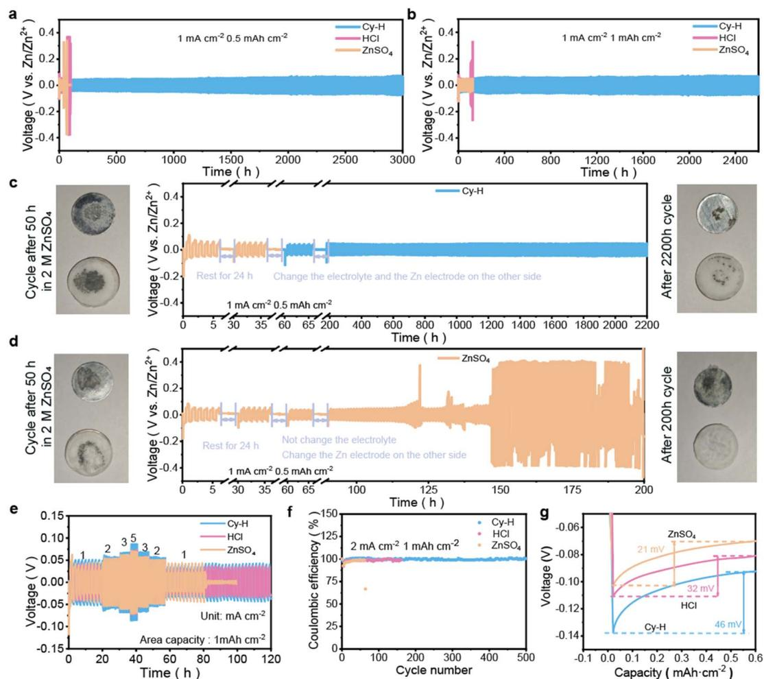
Fig. 3 Voltage profiles of Zn||Zn symmetric cells at (a) 0.5 and (b)  $1 \text{ mA h cm}^{-2}$ ; voltage profiles of Zn||Zn symmetric cells with Cy-H (c) and ZSO (d) for by-product elimination; (e) rate performance of Zn||Zn cells at different current densities; (f) CE of Cu||Zn asymmetric cells using different electrolytes; (g) nucleation overpotential of the first cycle of Zn||Cu asymmetric cells in different electrolytes.
