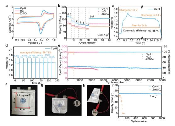
Fig. 5 CV curves (a) and rate performance (b) of  $Zn/I_2$  full cells with different electrolytes; self-discharge (c) and ten consecutive self-discharge tests (d); (e) long-term cycling performance of the  $Zn/I_2$  full cells at 2 A  $g^{-1}$ . Digital photograph of a pouch battery (f) and it powering a watch under normal (g) and flexed (h) conditions. (i) Long-term cycle performance at 1 A  $g^{-1}$  of assembled pouch batteries with different electrolytes.
