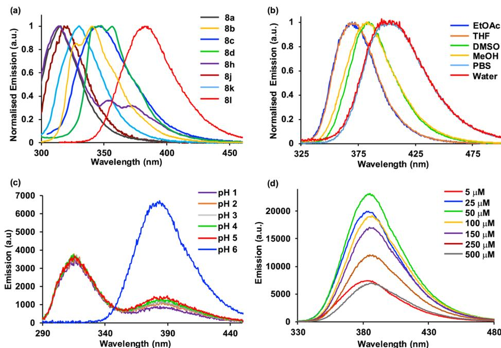
Fig. 2 (a) Normalised emission spectra of selected amino acids in methanol at 1–5  $\mu\text{M}$  (excitation was typically performed at absorption maxima). (b) Normalised emission spectra of **8l** at 5  $\mu\text{M}$  in various solvents. (c) Emission spectra of **8l** at 5  $\mu\text{M}$  at various pH. (d) Emission spectra of **8l** at various concentrations in methanol.
