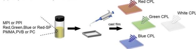
**Scheme 1** (a) Molecular structures of chiral helical PI, achiral fluorescein, multi-responsive achiral fluorescein, and polymer matrix. (b) Scheme of the preparation of composite films.
