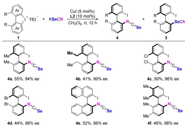
Scheme 5 Substrate scope of C–N coupling.<sup>a</sup> <sup>a</sup>Reaction conditions: cyclic diaryliodonium **1** (0.2 mmol, 1.0 equiv.), KSeCN (0.40 mmol, 2.0 equiv.), CuI (1.9 mg, 0.01 mmol, 5 mol%), L2 (7.0 mg, 0.02 mmol, 10 mol%) in CH<sub>2</sub>Cl<sub>2</sub> (5 mL) at 25 °C for 12 h. The ratios of **4** : **3** range from 1 : 1 to 1.5 : 1, see the ESI† for details.
