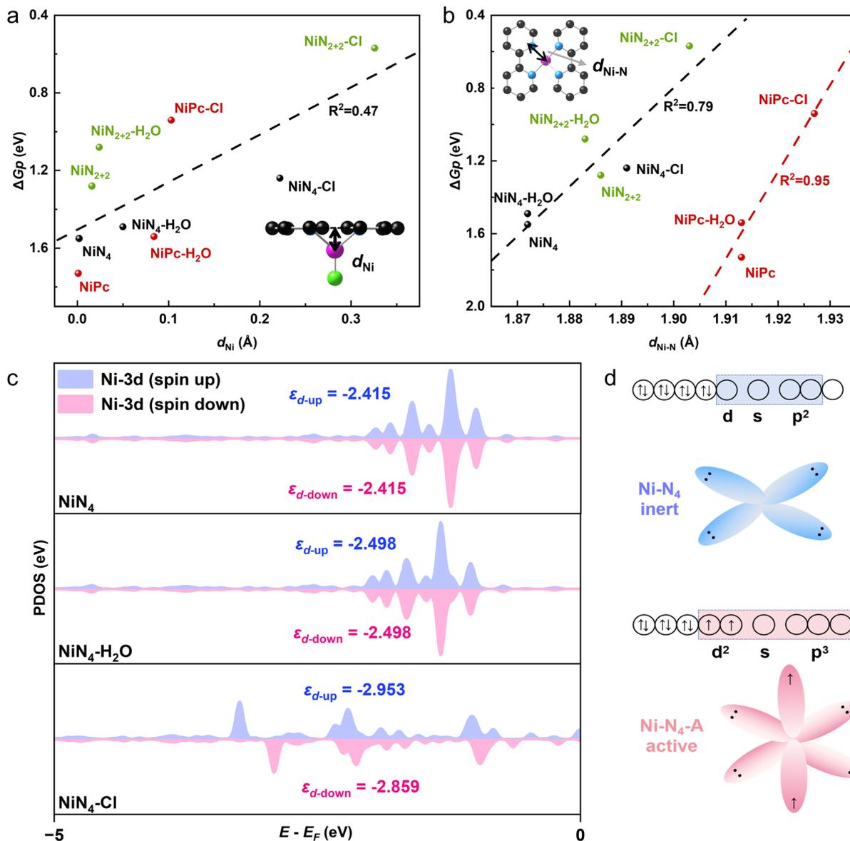
Fig. 4 The effect of Cl axial ligand on the geometric and electronic structure of Ni-N<sub>4</sub>. The relationship between  $\Delta G_p$  and (a)  $d_{Ni}$ , (b)  $d_{Ni-N}$ . (c) The partial density of states and d-band center of Ni atoms in NiN<sub>4</sub>, NiN<sub>4</sub>-Cl, and NiN<sub>4</sub>-H<sub>2</sub>O. (d) Schematic diagram of orbital hybridization of Ni atoms in Ni-N<sub>4</sub> with and without axial ligands.
