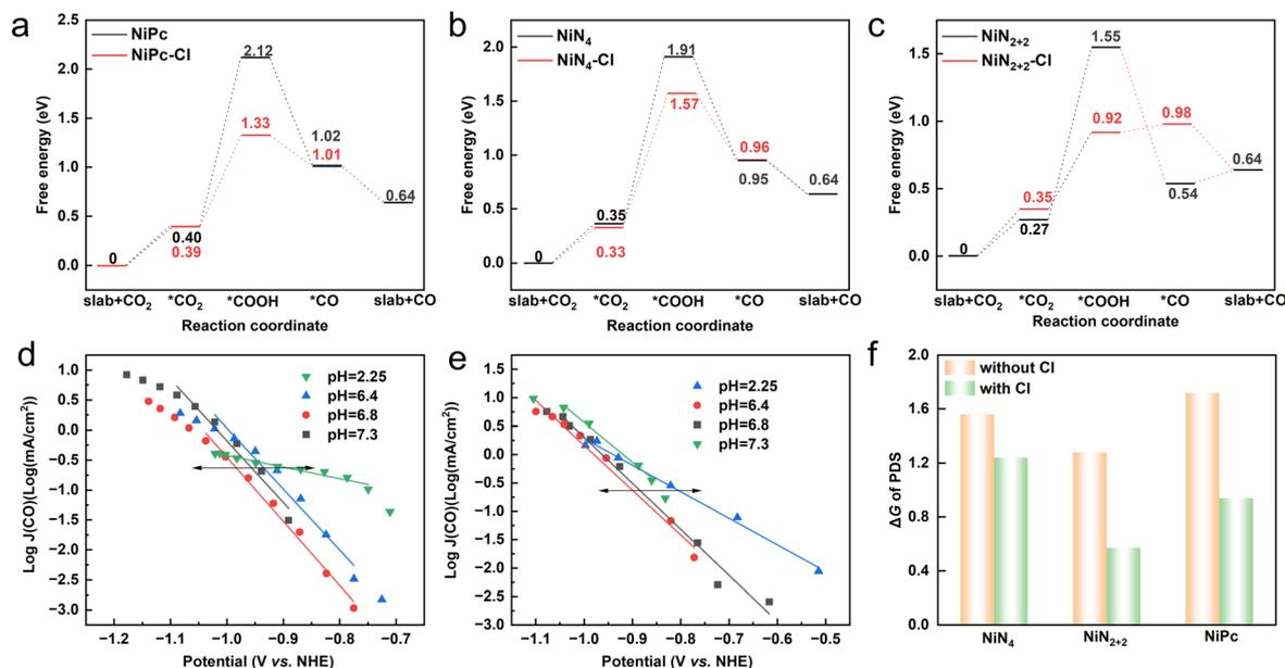
Fig. 2 The effect of Cl axial ligand on the energy barrier of PDS for the eCO<sub>2</sub>RR toward CO over Ni-N<sub>4</sub>. Free energy diagrams of the eCO<sub>2</sub>RR to CO for (a) NiPc, (b) NiN<sub>4</sub> and (c) NiN<sub>2+2</sub> with and without the Cl axial ligand. Experimental current densities plotted against potential vs. NHE for (d) NiPc and (e) Ni-N-C. (f) Comparison of the ΔG of PDS for NiPc, NiN<sub>4</sub> and NiN<sub>2+2</sub> with and without the Cl axial ligand.
