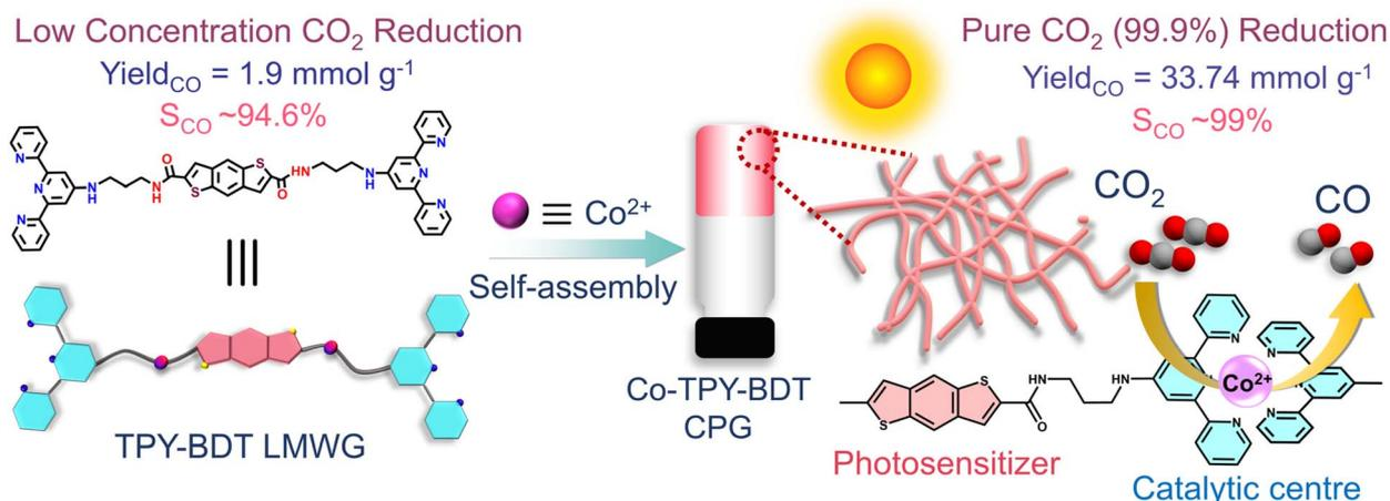
**Scheme 1** Schematic showing the self-assembly of the TPY-BDT LMWG with Co<sup>II</sup> to generate Co-TPY-BDT CPG with nanofiber morphology towards photocatalytic CO<sub>2</sub> reduction using pure CO<sub>2</sub> and low concentration CO<sub>2</sub>.
