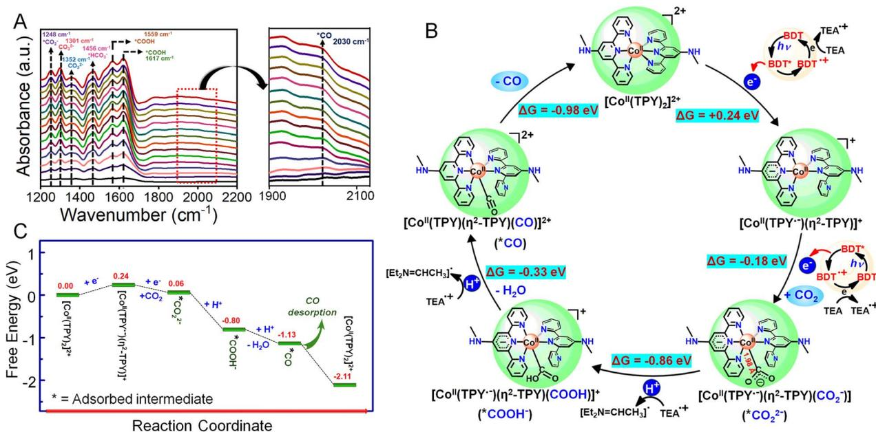
Fig. 4 (A) *In situ* DRIFT spectra of Co-TPY-BDT CPG under visible-light irradiation for CO formation. (B) Proposed mechanism for the reduction of CO<sub>2</sub> to CO utilizing the Co-TPY-BDT CPG catalyst. (C) Relative Gibbs free energy plot.
