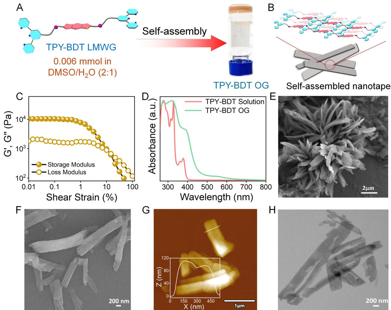
Fig. 1 (A) Schematic of the TPY-BDT LMWG towards the formation OG. (B) Schematic of the self-assembled nanotape morphology. (C) Strain sweep rheology measurement of TPY-BDT OG. (D) Comparison of absorption spectra of the TPY-BDT LMWG in solution with TPY-BDT OG in the xerogel state. (E and F) FESEM, (G) AFM, and (H) TEM images of TPY-BDT OG showing nanotape like morphology.
