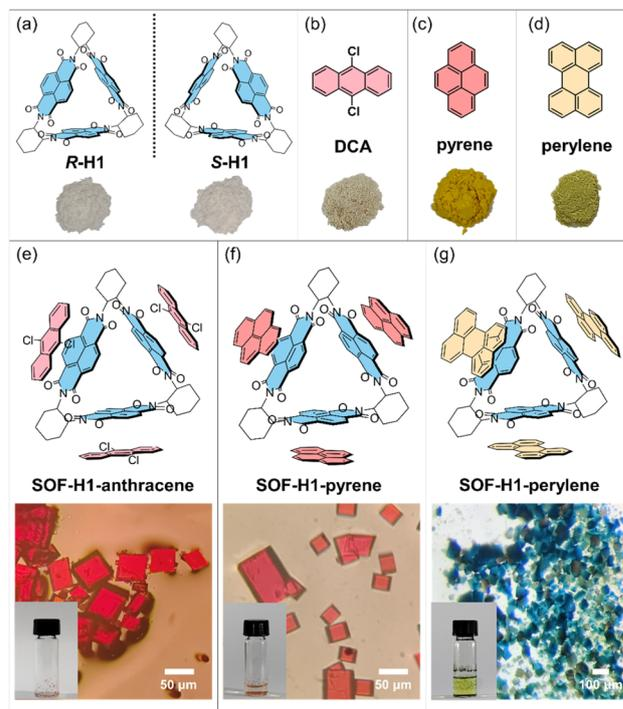
Fig. 1 (a) The chemical structures of the enantiomers of **H1** and their photographs. (b–d) The chemical structures of the guest molecules and their photographs. (e–g) The chemical structures of the three SOFs (SOF-**H1**-anthracene, SOF-**H1**-pyrene, and SOF-**H1**-perylene) and their optical microscope images and photographs. The *R* enantiomers were selected as representatives to present.
