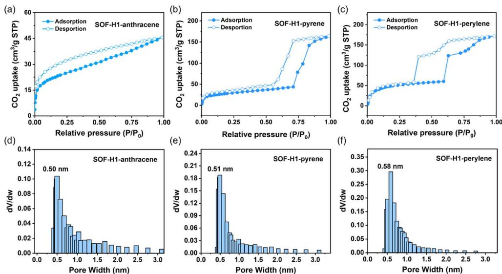
Fig. 4 CO<sub>2</sub> adsorption–desorption isotherms (195 K) of (a) SOF-H1-anthracene, (b) SOF-H1-pyrene, and (c) SOF-H1-perylene. Pore size distribution profiles of (d) SOF-H1-anthracene, (e) SOF-H1-pyrene, and (f) SOF-H1-perylene. The *R* enantiomers are selected as representatives.
