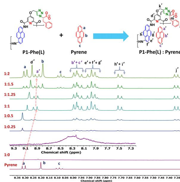
Fig. 3 A stacked plot of the <sup>1</sup>H NMR spectra (aromatic region) of pyrene, P1-Phe(*l*) (1 : 0), and P1-Phe(*l*) : pyrene (host-guest) complex, demonstrating the spectral changes upon addition of an increasing amount of pyrene to the polymer scaffold; a zoomed NMR spectra of the uncomplexed host polymer (1 : 0) has been depicted as the inset; <sup>1</sup>H NMR spectra were recorded in a mixture of DMSO-*d*<sub>6</sub> and triethylamine (TEA) (99.5 : 0.5) at 1 mM.
