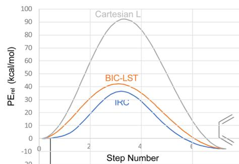
**Fig. 1** Comparison of Cartesian LST, BIC-LST and IRC for the conrotatory ring opening of cyclobutene at the M06-2X/cc-pVTZ level.
