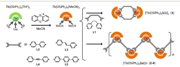
Scheme 1 The preparation of  $[Tb(OSiPh_3)_4Lx]_n$  [1 (n=2), L1 = 1,2-bis(4-pyridyl)ethane; 2, L2 = 4,4'-bipyridine; 3, L3 = 1,2-bis(4-pyridyl)ethene; 4, L4 = 1,2-bis(4-pyridyl)ethylene; 5, L5 = 1,4-bis(4-pyridyl)benzene].
