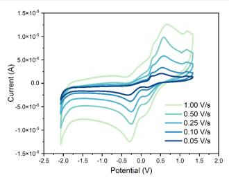
Fig. 4 Cyclic voltammograms of 1 (1.0 mM in dichloromethane) with  $n\text{-Bu}_4\text{NPF}_6$  (0.1 mM) as the supporting electrolyte at a sweep rate of 500 mV s<sup>-1</sup> versus Fc/Fc<sup>+</sup>.
