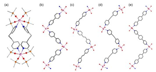
Fig. 1 The crystal structures of 1 (a), 2 (b), 3 (c), 4 (d), and 5 (e). Simplified views of the  $Ph_3SiO^-$  ligands (O, Si, and the Si-bound C atoms in 1, and O atoms only in 2–5) are shown with the bridging ligands (hydrogen atoms are removed for clarity) and the Tb(v) centers (color legends: Tb, lilac; O, red; C, grey; N, blue; Si, orange).
