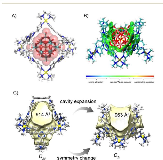
Fig. 2 (A) Crystal structure of  $(\text{SiMo}_{12}\text{O}_{40}) \subset 2 \cdot (\text{NO}_3)_8$ . (B) Visualized intermolecular binding iso-surface between **2** and  $\text{SiMo}_{12}\text{O}_{40}^{4-}$  ( $\delta g_{\text{inter}} = 0.003$ ). (C) Cavity volumes of cage **1** and bowl **2** calculated using the MoloVol program based on the crystal structures.
