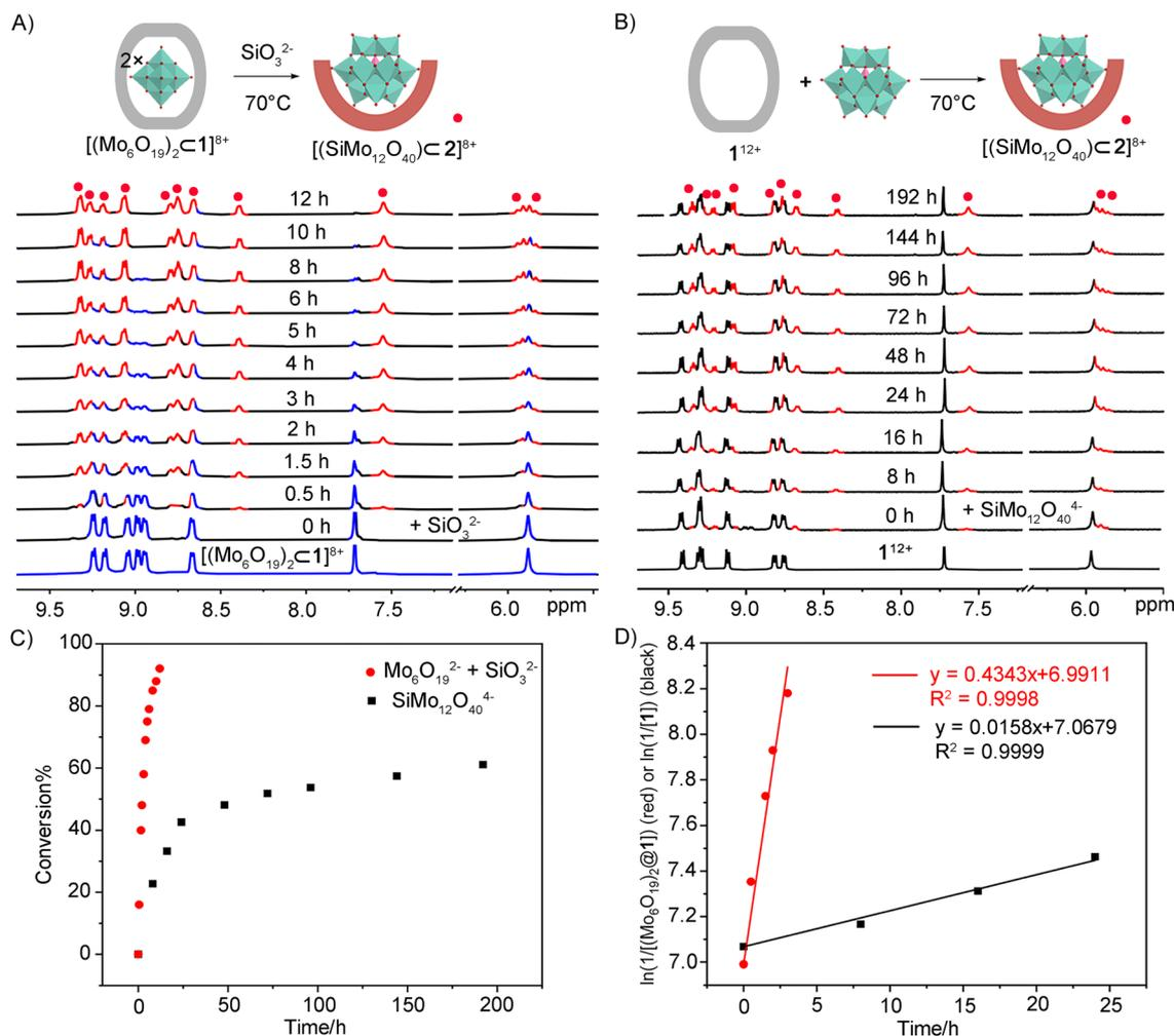
Fig. 3 Time-dependent  $^1\text{H}$  NMR (400 M,  $\text{D}_2\text{O}$ , 298 K) for (A)  $(\text{Mo}_6\text{O}_{19})_2 \subset 1 \cdot (\text{NO}_3)_8$  after adding 1 equiv. of  $\text{Na}_2\text{SiO}_3$  and heating at  $70^\circ\text{C}$  and (B) the  $\text{SiMo}_{12}\text{O}_{40}^{4-}$  induced structural transformation from 1 to 2. (C) Conversion and (D) pseudo-first-order kinetic plots for the above two cage transformation reactions.
