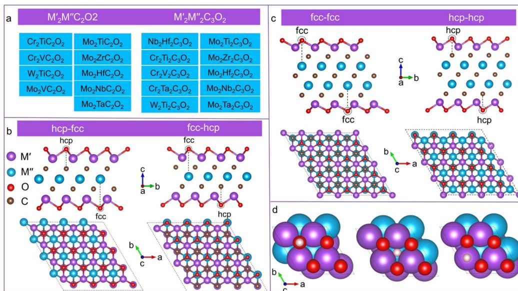
**Fig. 3** Crystal structures. (a) List of 9  $M'_2M''C_2O_2$  and 10  $M'_2M''C_3O_2$ , demonstrated to be synthesizable, stable and conductive, are investigated in this work for the HER. (b and c) Atomic structures of  $M'_2M''C_2O_2$  in hcp-fcc and fcc-hcp types and  $M'_2M''C_3O_2$  in fcc-fcc and hcp-hcp types viewed from the top and side, respectively. (d) Top view of three distinct adsorption structures for 1/4 hydrogen coverage on MXenes.
