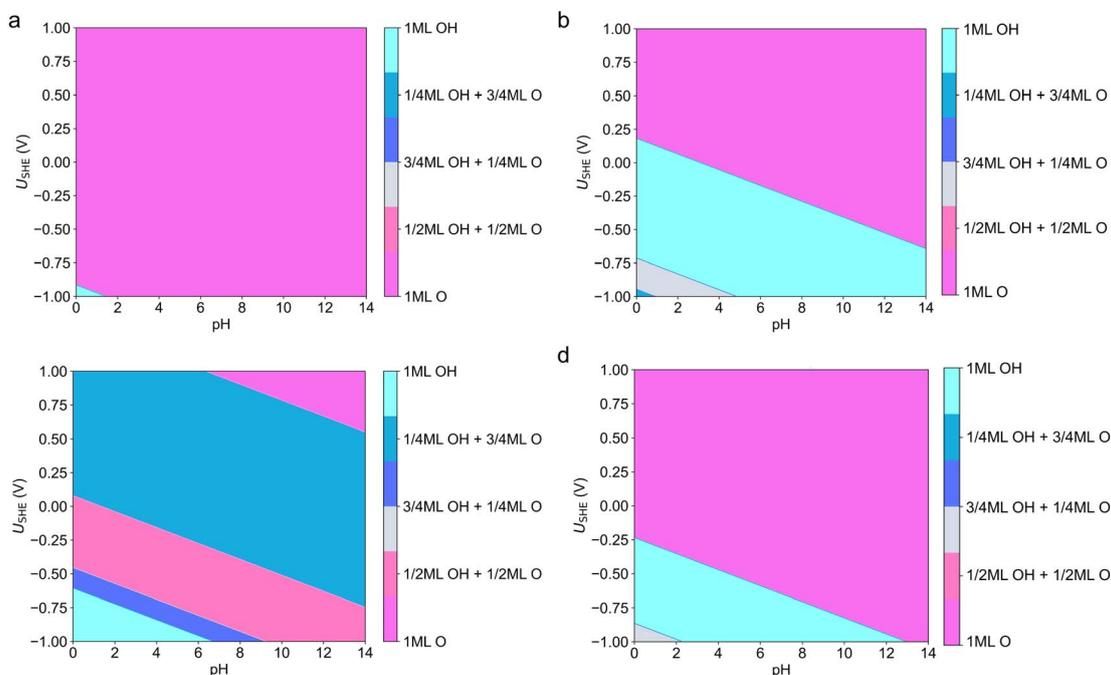
Fig. 2 Surface Pourbaix diagrams of (a)  $Cr_2TiC_2$ , (b)  $Mo_2TiC_2$ , (c)  $Ti_2Ta_2C_3$  and (d)  $W_2Hf_3C_2$ . The most thermodynamically stable states of the surface under relevant  $U_{SHE}$  conditions and pH values are labeled by the terminations.
