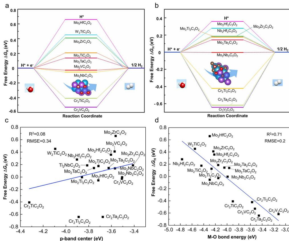
Fig. 5 (a and b) HER free energy diagrams of  $M'_2M''C_2O_2$  and  $M'_2M''C_3O_2$  under standard conditions, respectively. (c and d) Relationships between  $\Delta G_{\text{H}}$  and descriptors including (c) the p-band center of the oxygen functional group and (d) the bond energy between the first-layer transition metal and oxygen of different MXene systems, respectively.
