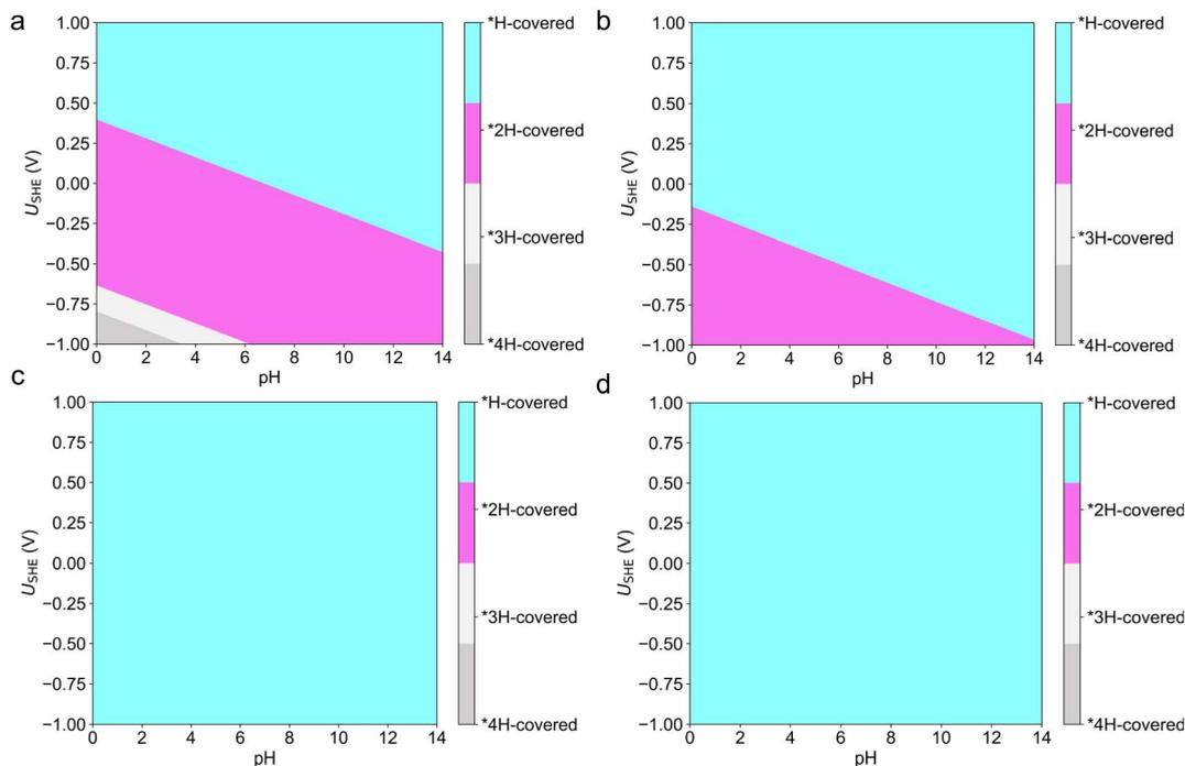
**Fig. 4** The surface Pourbaix diagrams as a function of pH and potential under different hydrogen coverage. Surface Pourbaix diagrams of (a)  $Cr_2TiC_2O_2$ , (b)  $Mo_2TiC_2O_2$ , (c)  $W_2Hf_2C_3O_2$  and (d)  $W_2Zr_2C_3O_2$ .
