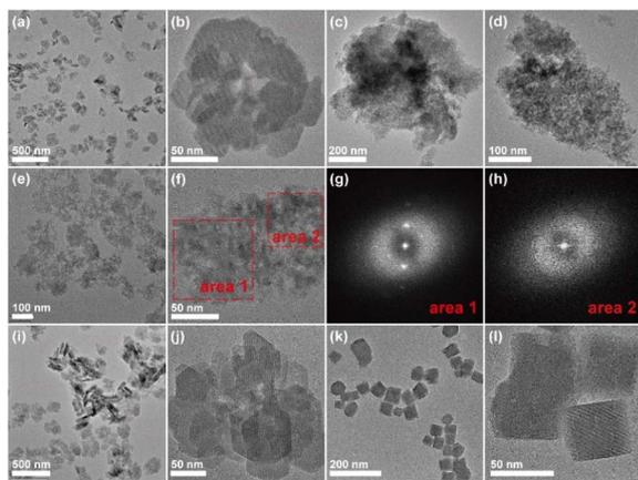
**Fig. 1** (a) Low and (b) high magnification TEM images of TS-1-E-80-170. TEM images of TS-1-E-80-170 crystallized at 80 °C for 48 h and then at 170 °C for (c) 3 h and (d) 6 h, (e and f) 10 h, and (i and j) 48 h. (g and h) FFT diffractograms of area 1 and area 2 in (f). (k) Low and (l) high magnification TEM images of TS-1-C-80-170 crystallized at 80 °C for 48 h and then at 170 °C for 48 h.
