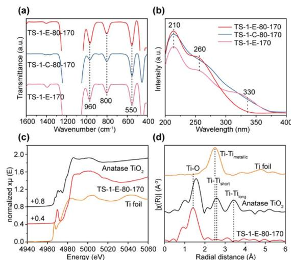
**Fig. 2** (a) FT-IR spectra and (b) UV-vis spectra of TS-1-E-80-170, TS-1-C-80-170, and TS-1-E-170. (c) Ti K-edge XANES spectra and (d) Fourier transform  $k^2$ -weighted Ti EXAFS spectra in  $R$ -spacing of TS-1-E-80-170, anatase, and Ti foil reference.
