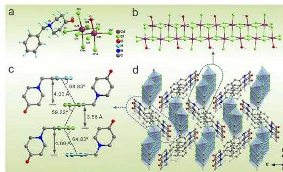
Fig. 1 (a) Asymmetric unit and (b) inorganic polyanionic [Cd<sub>2</sub>Cl<sub>5</sub>H<sub>2</sub>O]<sub>*n*</sub><sup>*n*-</sup> chain of NBP-Cd. (c) Ladder-type arrangement of organic cations. (d) 3D stacking diagram along the *a* axis.
