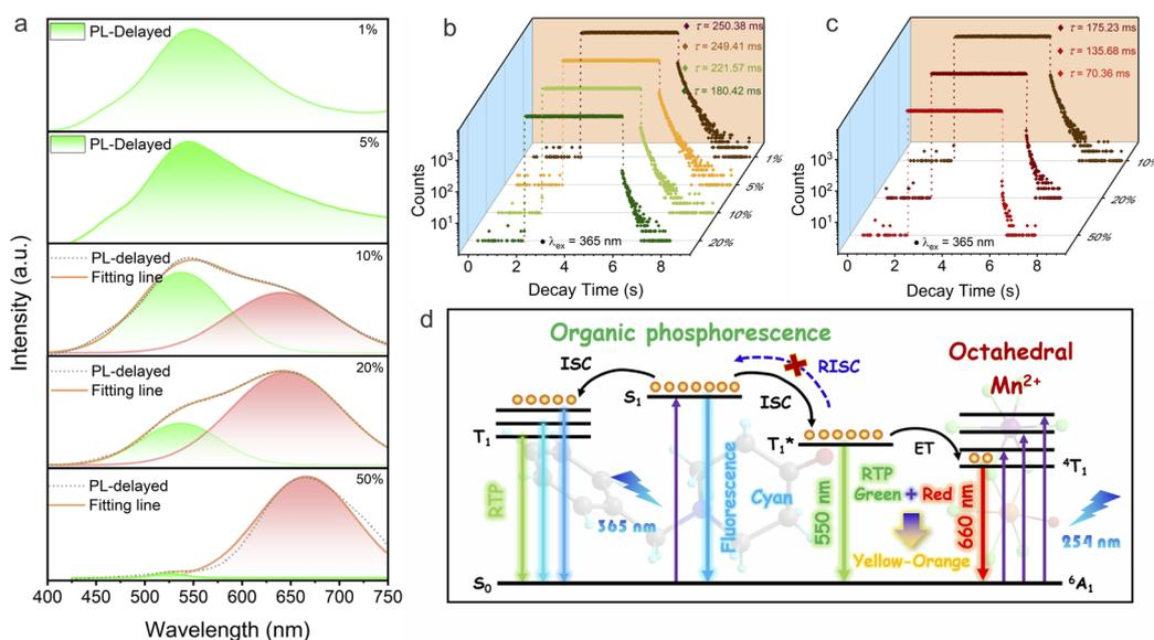
Fig. 6 (a) Delayed emission spectra and corresponding kinetic decay curves of emission peaks at (b) 550 nm and (c) 660 nm in NBP-Cd: $x\text{Mn}^{2+}$  under 365 nm excitation. (d) Schematic illustration of the proposed mechanism for the  $\text{Mn}^{2+}$  doped NBP-Cd system.
