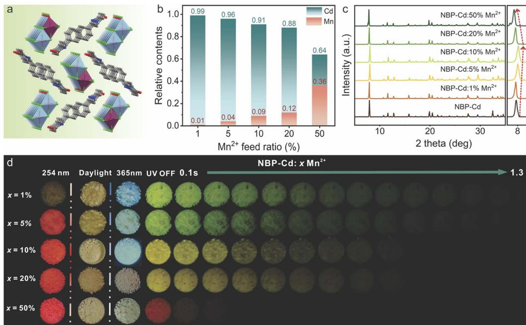
Fig. 4 (a) Schematic representation of the crystal structure of NBP-Cd: $x\text{Mn}^{2+}$ . (b) Actual  $\text{Mn}^{2+}$  content as a function of feed ratio of Mn and Cd in doped NBP-Cd systems. (c) PXRD patterns of NBP-Cd: $x\text{Mn}^{2+}$  samples. (d) Photographs of NBP-Cd: $x\text{Mn}^{2+}$  crystals under 254 nm and 365 nm irradiations as well as after removing 365 nm irradiation.
