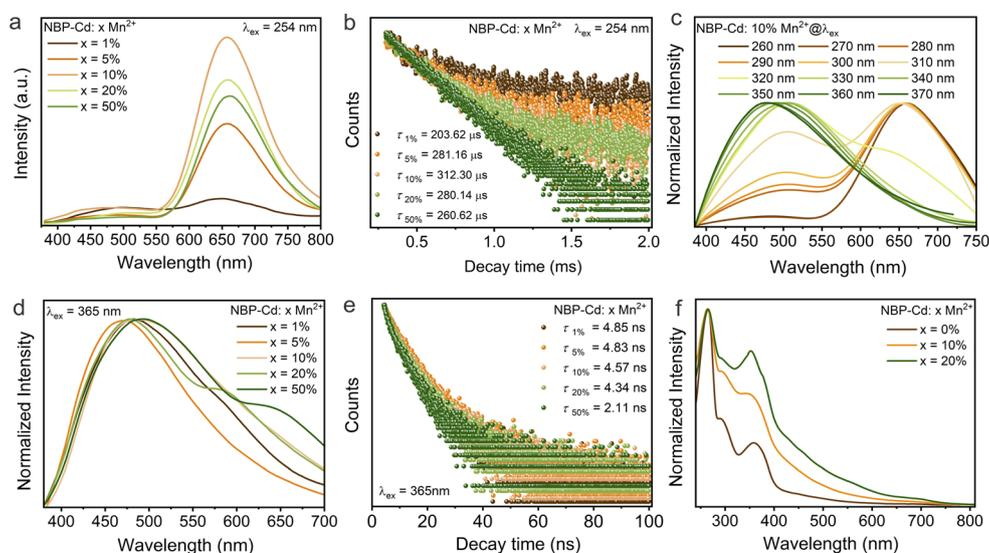
Fig. 5 (a) Prompt emission spectra and (b) corresponding decay curves for the red emissions at 660 nm in NBP-Cd: $x\text{Mn}^{2+}$  under excitation at 254 nm. (c) Excitation-dependent emission spectra of the NBP-Cd:10%Mn<sup>2+</sup> sample. (d) Prompt emission spectra and (e) corresponding decay curves for high-energy yellow-green emissions in NBP-Cd: $x\text{Mn}^{2+}$  under excitation at 365 nm. (f) UV-vis absorption spectra of NBP-Cd: $x\text{Mn}^{2+}$  ( $x = 0, 10\%$ , and  $20\%$ ).
