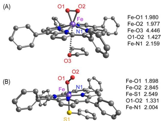
Fig. 7 Optimized geometries of (A) [(THF)(TPP)Fe<sup>III</sup>(O<sub>2</sub><sup>2-</sup>)]<sup>-</sup>, and (B) [(ArS<sup>-</sup>)(TPP)Fe<sup>III</sup>(O<sub>2</sub><sup>2-</sup>)]<sup>2-</sup> with calculated bond lengths shown in Å.
