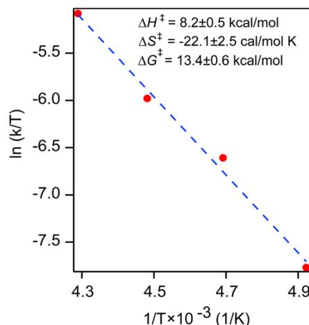
**Fig. 5** Eyring analysis data showing the dependence of ln( $k/T$ ) on  $1/T$  for the reaction between a 50  $\mu$ M solution of [(ArO<sup>-</sup>)(TPP)Fe<sup>III</sup>(O<sub>2</sub><sup>2-</sup>)]<sup>2-</sup> and acetophenone oxime at -40, -50, -60 and -70 °C. Solvent = 9 : 1 DCM : THF.
