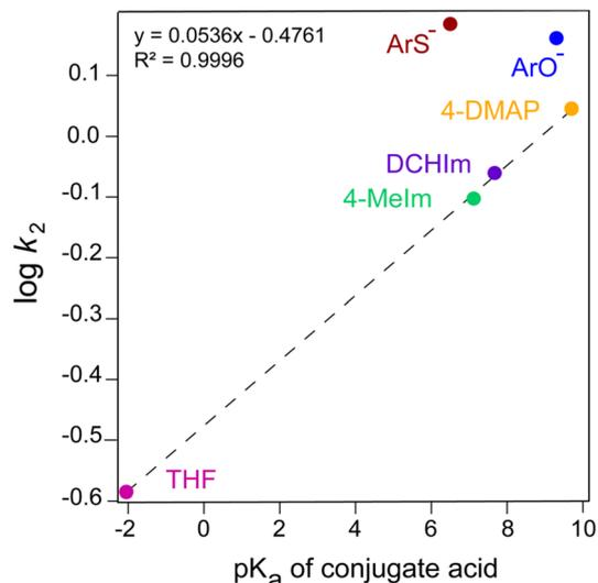
**Fig. 4** The correlation between log  $k_2$  values for [(B)(TPP)Fe<sup>III</sup>(O<sub>2</sub><sup>2-</sup>)]<sup>-</sup> mediated acetophenone oxime oxidation reactions (in 9 : 1 DCM : THF at -40 °C) and the pK<sub>a</sub> values of conjugate acids of the axially ligating B ligands, where B = THF (magenta), 4-MeIm (green), DCHIm (purple), 4-DMAP (orange), ArO<sup>-</sup> (blue) and ArS<sup>-</sup> (brick red).
