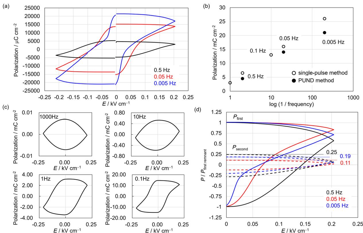
Fig. 3 (a) Polarization–electric field hysteresis loops obtained *via* PUND measurements. (b) Polarization as a function of frequency. (c) Frequency dependency on the hysteresis loops. (d) Frequency dependency on the polarization behavior of the first and second pulses. The vertical axis is the ratio of the polarization of the first or second pulse and the remnant polarization value of the first pulse.  $P_{\text{first or second}} = I_{\text{first or second pulse}} \times t$ .
