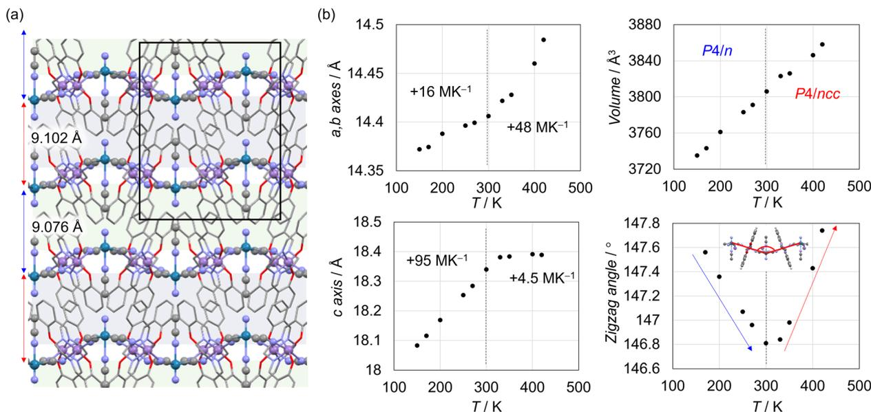
Fig. 6 (a) Crystal structure of  $\text{MnReMeCN}_{\text{LT}}$  ( $P4/n$ ) at 200 K. The black square indicates the unit cell. (b) Results of the thermal expansion behavior of  $\text{MnReMeCN}$  in terms of the thermal variation of the cell parameters, cell volume, and angles between the tetracyanomethylate units in the zigzag layer.
