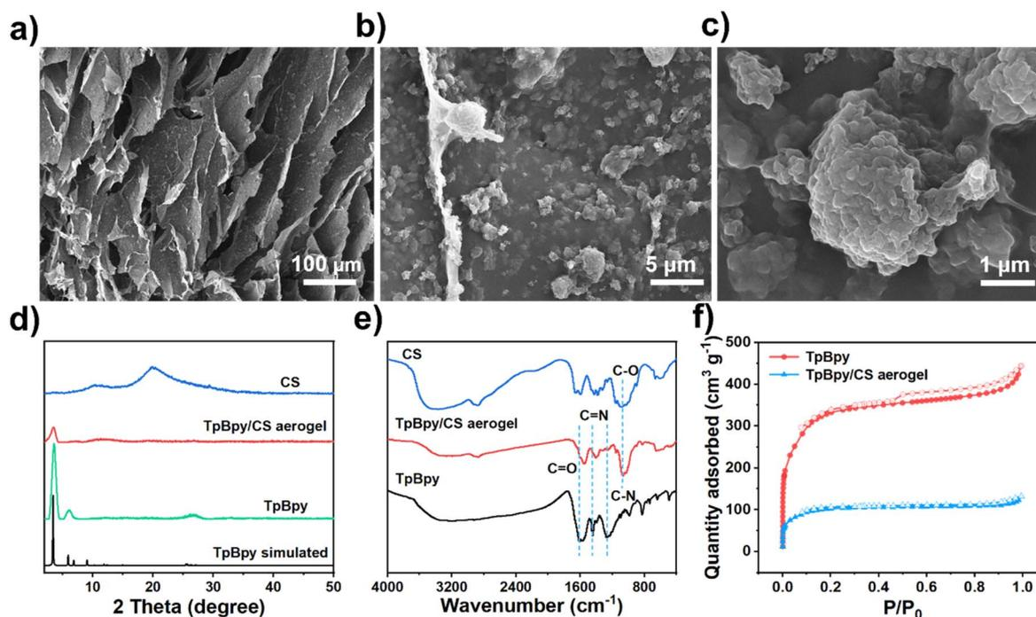
Fig. 1 (a–c) SEM micrographs of TpBpy/CS aerogel; (d) XRD patterns and (e) FT-IR spectra of CS, TpBpy, and TpBpy/CS aerogel; (f)  $\text{N}_2$  adsorption–desorption isotherms of TpBpy/CS aerogel and TpBpy.
