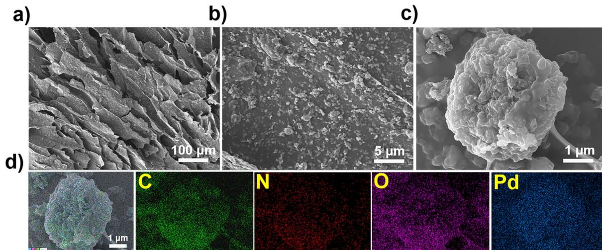
Fig. 3 (a–c) Pd(II)-loaded TpBpy/CS aerogel; (d) SEM micrographs and the corresponding EDS mapping images of Pd(II)-loaded TpBpy/CS aerogel.
