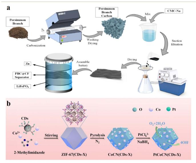
Fig. 12 (a) Schematic illustration depicting the preparation process of PBC@CF-separators and their application in an aqueous Zn-LiFePO<sub>4</sub> dual ion full battery; Reproduced with permission. <sup>147</sup> Copyright 2022, Elsevier. (b) Schematic diagram of the formation of the PtCoCN (CDs-X) catalyst. Reproduced with permission. 148 Copyright 2024, Royal Society of Chemistry.
