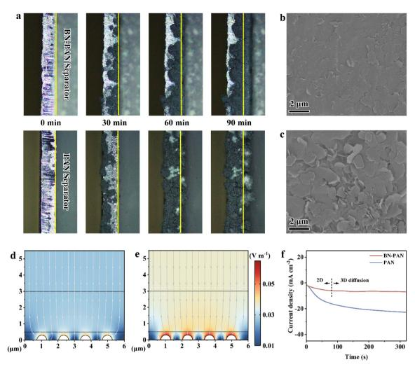
Fig. 3 The Zn plating/stripping process in Zn//Zn cells. (a) In situ optical microscope images of Zn plating/stripping at 5 mA for Zn anodes with the use of BN-PAN and PAN separators. The SEM images of the Zn anode surface after 10 cycles with the (b) BN-PAN separator and (c) PAN separator. The electrical field models based on the (d) BN-PAN separator and (e) PAN separator. (f) The amperometric i-t curves of Zn//Zn cells with BN-PAN and PAN separators at an overpotential of -150 mV.
