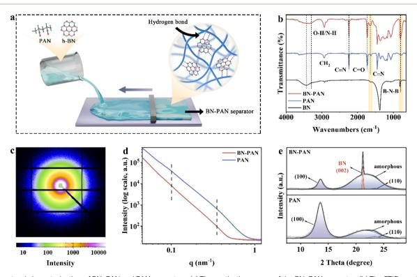
Fig. 1 Structural characterization of BN-PAN and PAN separators. (a) The synthetic process of the BN-PAN separator. (b) The FTIR spectra of the BN-PAN separator, the PAN separator and BN. (c) 2D SR-SAXS pattern of the BN-PAN separator. (d) Corresponding 1D integrated curves of the 2D SR-SAXS patterns of the BN-PAN separator and PAN separator. (e) Multipeak fitting of the 1D integrated WAXS curve of the BN-PAN separator and PAN separator.
