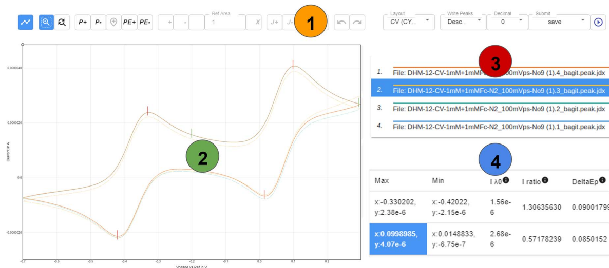
Fig. 4 General schematic overview of the different information/action panels of a CV layout in ChemSpectra . Additional metadata such as scan rate, solvent and others are not described here and are part of the metadata section (see ESI†). (1) Action panel that allows to select and switch between different actions (e.g. peak picking); (2) the plotting area shows all cycles and highlights the one selected in area (3); (3) the graph selection area can be used to select a single cycle (out of different ones given in the plot); (4) for a selected sweep, the picked minima and maxima are summarized in a table form and used for the calculation of i_{pa}/i_{pc} , E_{1/2} and \Delta E_p . The different panels (1–4) were selected from a screenshot of ChemSpectra and the ratio of size was changed for a clearer representation.
