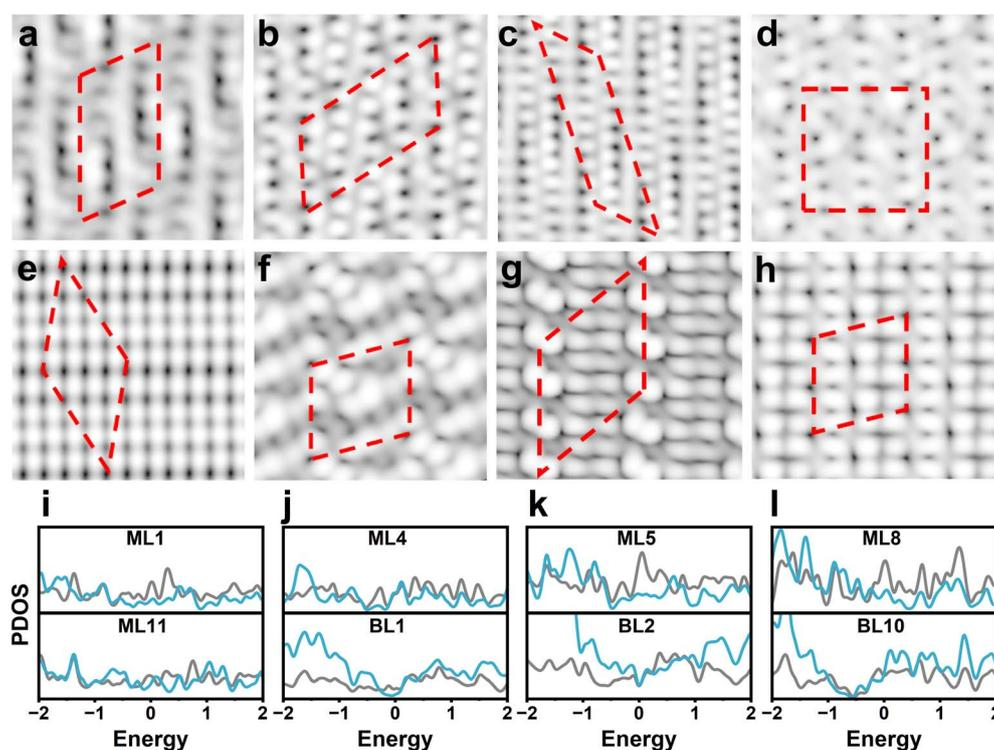
**Fig. 5** Simulated images of (a) ML1, (b) ML4, (c) ML5, (d) ML8, (e) ML11, (f) BL1, (g) BL2, and (h) BL5 on Ag(100). The red dashed lines denote the primitive cell. The (i)–(l) corresponding projected density of states, in which the gray and cyan lines denote Ag and B atoms, respectively. The Fermi energy level is set as 0 eV.
