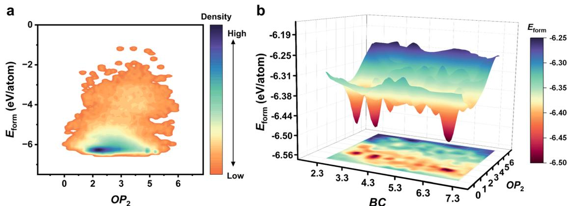
Fig. 2 (a) Illustration of the global dataset from first principles for borophene on Ag(100) systems shown as a contour map of formation energy ( $E_{\text{form}}$ ) vs.  $OP_2$ . The density is indicated by color. The  $OP_2$  parameter reflects the averaged geometrical environment of bonded boron atoms. (b) Schematic diagram of the potential energy surface (PES) for borophene on Ag(100) systems scaled by BC and  $OP_2$  dimensionality.
