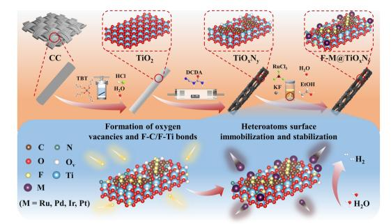
Fig. 1 An in situ fluoride ion etching and heteroatoms immobilization strategy for the synthesis of  $F-M@TiO_xN_v$  (M = Ru, Pd, Ir, Pt) (schematic).
