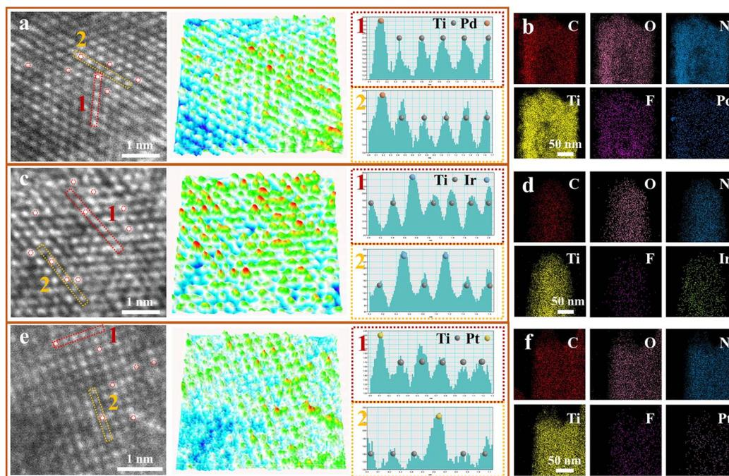
Fig. 5 HRTEM images and related lattice pseudo-colour surface intensity plot and X-Y intensity profiles of (a) F-Pd@TiO<sub>x</sub>N<sub>y</sub>, (c) F-Ir@TiO<sub>x</sub>N<sub>y</sub> and (e) F-Pt@TiO<sub>x</sub>N<sub>y</sub>. STEM-EDS mapping images of (b) F-Pd@TiO<sub>x</sub>N<sub>y</sub>, (d) F-Ir@TiO<sub>x</sub>N<sub>y</sub> and (f) F-Pt@TiO<sub>x</sub>N<sub>y</sub>.
