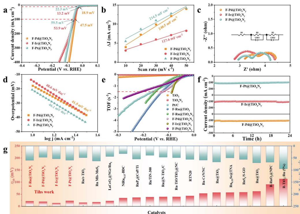
Fig. 6 (a) LSV polarization curves, (b) calculated ECSA, (c) Nyquist plots, (d) Tafel slope, (e) calculated TOF curves and (f) long-term durability at 100 mA cm<sup>-2</sup> of F-Pd@TiO<sub>x</sub>N<sub>y</sub>, F-Ir@TiO<sub>x</sub>N<sub>y</sub> and F-Pt@TiO<sub>x</sub>N<sub>y</sub>. (g) Comparison of the overpotentials at 10 mA cm<sup>-2</sup> and Tafel values of F-M@TiO<sub>x</sub>N<sub>y</sub> (M = Ru, Pd, Ir, Pt) with state-of-the-art Ru-based electrocatalysts in an alkaline electrolyte.
