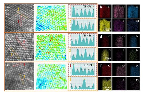
Fig. 5 HRTEM images and related lattice pseudo-colour surface intensity plot and X-Y intensity profiles of (a)  $F-Pd@TiO_xN_y$ , (c)  $F-Ir@TiO_xN_y$  and (e)  $F-Pt@TiO_xN_v$ . STEM-EDS mapping images of (b)  $F-Pt@TiO_xN_v$ , (d)  $F-Ir@TiO_xN_v$  and (f)  $F-Pt@TiO_xN_v$ .
