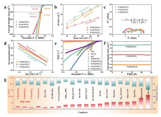
Fig. 6 (a) LSV polarization curves, (b) calculated ECSA, (c) Nyquist plots, (d) Tafel slope, (e) calculated TOF curves and (f) long-term durability at 100 mA cm $^{-2}$  of F-Pd@TiO<sub>x</sub>N<sub>y</sub>, F-Ir@TiO<sub>x</sub>N<sub>y</sub> and F-Pt@TiO<sub>x</sub>N<sub>y</sub>. (g) Comparison of the overpotentials at 10 mA cm $^{-2}$  and Tafel values of F- $M@TiO_xN_v$  (M = Ru, Pd, Ir, Pt) with state-of-the-art Ru-based electrocatalysts in an alkaline electrolyte.
