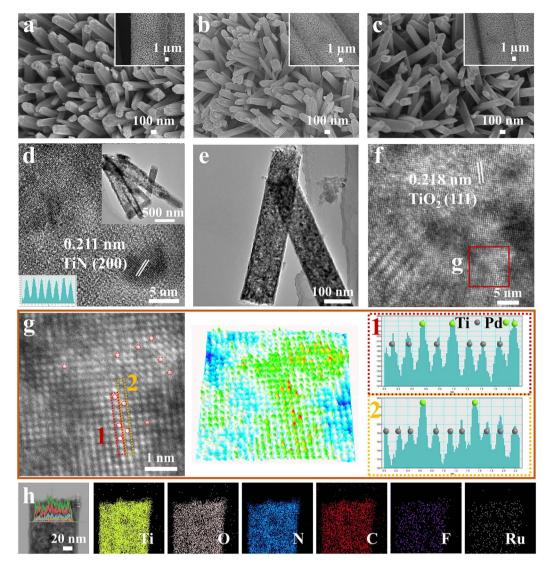
Fig. 2 SEM images of (a)  $TiO_2$ , (b)  $TiO_xN_y$  and (c)  $F-Ru@TiO_xN_y$  composites. TEM images of (d)  $TiO_xN_y$  (inset is a TEM image and lattice fringe of  $TiO_xN_v$ ) and (e and f) F-Ru@ $TiO_xN_v$ . (g) HRTEM image and related lattice pseudo-colour surface intensity plot and X-Y intensity profiles of F-Ru@TiO<sub>x</sub>N<sub>v</sub>. (h) STEM-EDS line scan and mapping images of F-Ru@TiO<sub>x</sub>N<sub>v</sub>.
