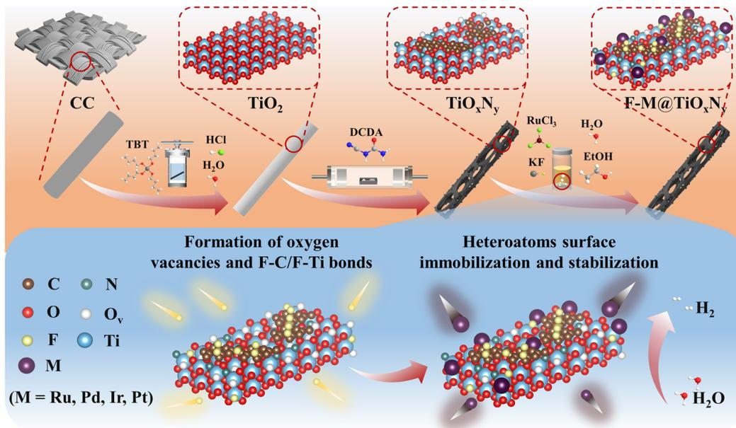
Fig. 1 An *in situ* fluoride ion etching and heteroatoms immobilization strategy for the synthesis of F-M@TiO<sub>x</sub>N<sub>y</sub> (M = Ru, Pd, Ir, Pt) (schematic).
