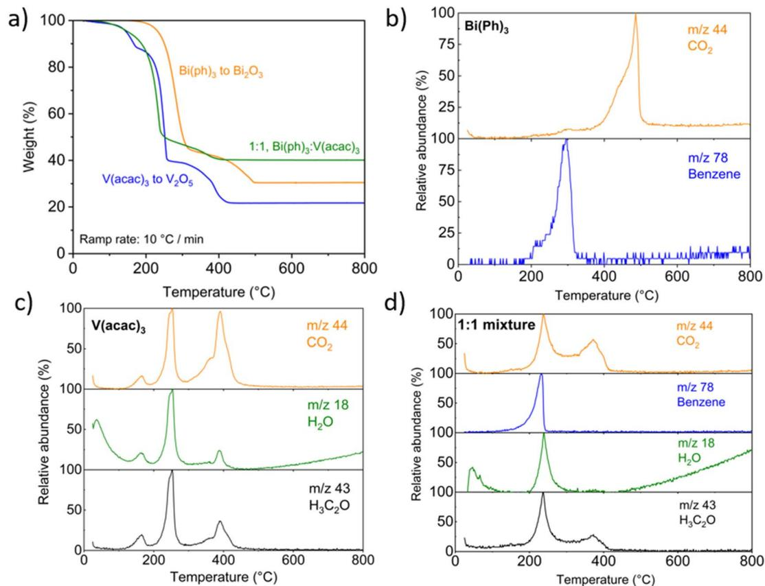
Fig. 2 TGA-mass spectrometry (MS) of the precursors used in the AACVD synthesis of  $\text{BiVO}_4$  (a) weight loss % as a function of temperature, and mass spectrometry of volatile materials for (b)  $\text{Bi}(\text{Ph})_3$ , (c)  $\text{V}(\text{acac})_3$ , and (d) 1 : 1 mixture of  $\text{Bi}(\text{Ph})_3$  and  $\text{V}(\text{acac})_3$ .
