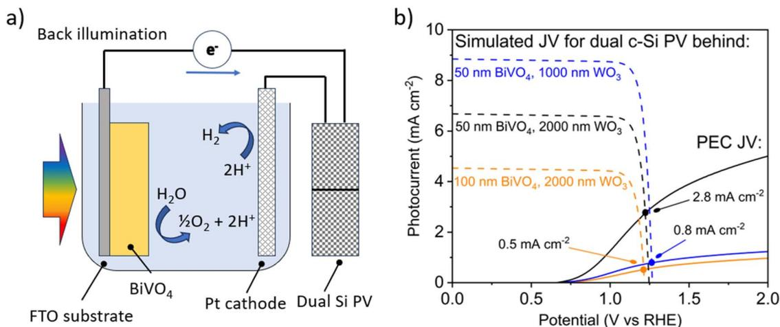
Fig. 11 (a) Schematic of the hypothetical PV-PEC device with a dual c-Si PV electrically in series and optically in tandem with a back-illuminated PEC photoanode, (b)  $J$ - $V$  curves for samples as indicated under back illumination as solid lines, and simulated  $J$ - $V$  curves of corresponding dual c-Si PV modules behind the PEC module as dashed lines. Simulations and measured curves are calibrated to AM1.5G 1 sun illumination.
