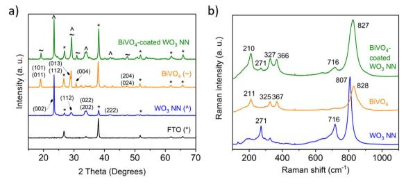
Fig. 4 (a) XRD patterns and (b) Raman spectra for 1000 nm long  $WO_3$  nanoneedles,  $BiVO_4$  and 50 nm thick  $BiVO_4$  coated on  $WO_3$  nanoneedles corresponding to monoclinic  $WO_3$  (ref. 34, 48 and 49) and monoclinic  $BiVO_4$ .
