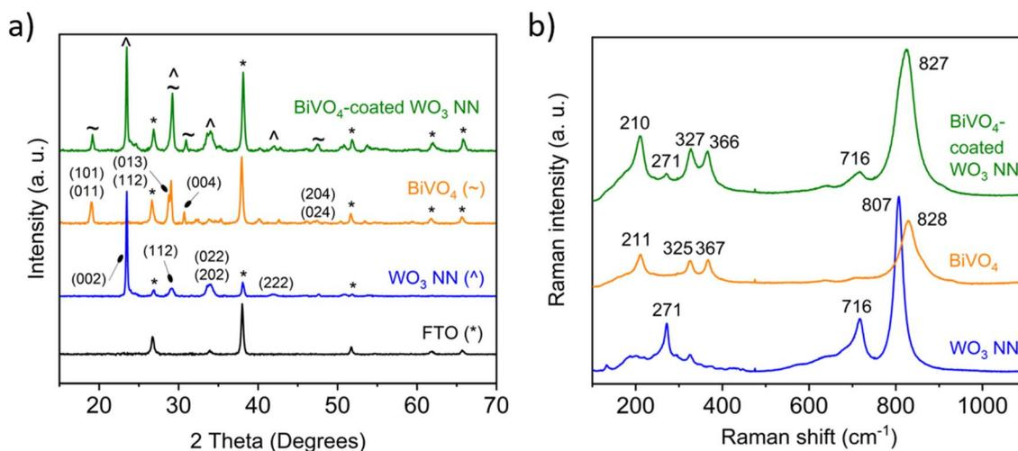
Fig. 4 (a) XRD patterns and (b) Raman spectra for 1000 nm long  $\text{WO}_3$  nanoneedles,  $\text{BiVO}_4$  and 50 nm thick  $\text{BiVO}_4$  coated on  $\text{WO}_3$  nanoneedles corresponding to monoclinic  $\text{WO}_3$  (ref. 34, 48 and 49) and monoclinic  $\text{BiVO}_4$ .<sup>50,51</sup>
