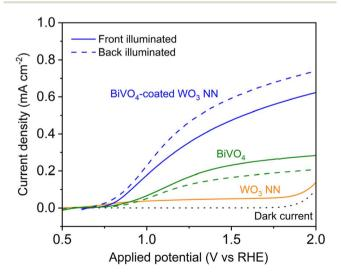
Fig. 7 J-V curves for 1000 nm thick WO $_3$  NN (pH 1.1, 0.1 M H $_2$ SO $_4$  (aq.)), 200 nm thick BiVO $_4$  and 50 nm thick BiVO $_4$ -coated 1000 nm thick WO $_3$  NN (pH 7, 0.1 M K $_2$ HPO $_4$ /KH $_2$ PO $_4$  (aq.)) on TEC15 FTO-coated glass. Scan rate: 10 mV s $^{-1}$ , illuminated with a 75 W Xe lamp attenuated with a neutral density filter at approximately 1 sun intensity. Solid lines represent front illumination, and dashed lines represent back illumination.
