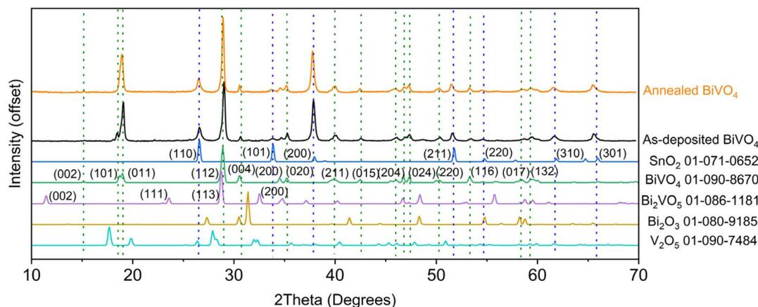
Fig. 3 XRD patterns for  $\text{BiVO}_4$  films grown on FTO-coated glass by AACVD before annealing (as deposited) and after annealing at 500 °C for 2 hours in air. Data is plot alongside PDF card references patterns for  $\text{SnO}_2$  (i.e. the FTO substrate),  $\text{BiVO}_4$ ,  $\text{Bi}_2\text{VO}_5$ ,  $\text{Bi}_2\text{O}_3$  and  $\text{V}_2\text{O}_5$ .
