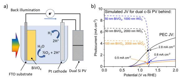
Fig. 11 (a) Schematic of the hypothetical PV-PEC device with a dual c-Si PV electrically in series and optically in tandem with a back-illuminated PEC photoanode, (b) J-V curves for samples as indicated under back illumination as solid lines, and simulated J-V curves of corresponding dual c-Si PV modules behind the PEC module as dashed lines. Simulations and measured curves are calibrated to AM1.5G 1 sun illumination.
