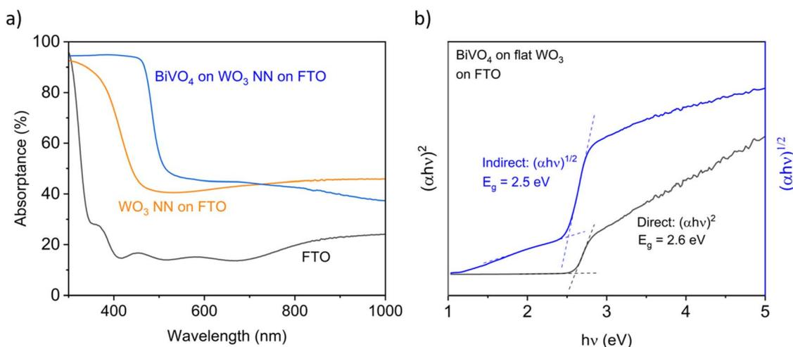
Fig. 5 (a) UV-vis absorbance for 2000 nm thick  $\text{WO}_3$  NN and 100 nm  $\text{BiVO}_4$ -coated NN  $\text{WO}_3$  compared to FTO-coated glass and (b) Tauc plots derived from measurements of transmittance and total reflectance of 400 nm planar  $\text{BiVO}_4$  on 100 nm planar  $\text{WO}_3$  on FTO-coated glass.
