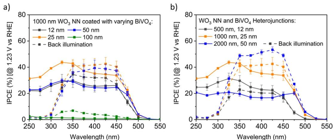
Fig. 8 Exemplar IPCE profiles for BiVO<sub>4</sub>-coated WO<sub>3</sub> on FTO, measured at pH 7 in 0.1 M KH<sub>2</sub>PO<sub>4</sub>/K<sub>2</sub>HPO<sub>4</sub> (aq.) buffer electrolyte under front and back illumination (dashed lines), with 95% confidence intervals for triplicate measurements (a) varying BiVO<sub>4</sub> on 1000 nm long WO<sub>3</sub> nanoneedles, and (b) constant ratio of varying BiVO<sub>4</sub> and WO<sub>3</sub> nanoneedle thicknesses.
