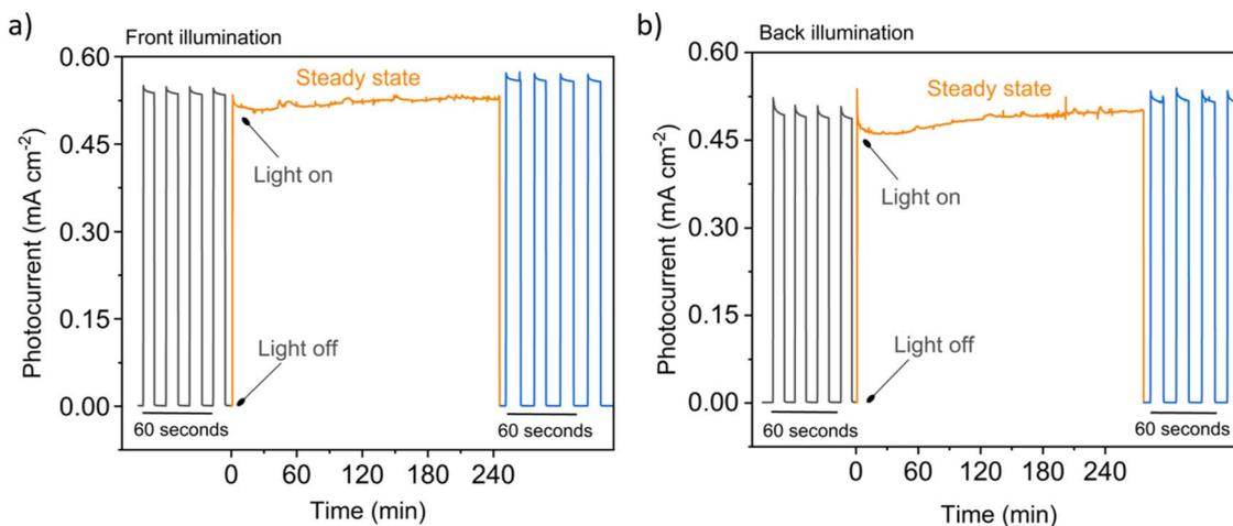
Fig. 9 Chronoamperometry stability measurements of a representative 500 nm long WO<sub>3</sub>/50 nm thick BiVO<sub>4</sub> heterojunction photoanode illuminated with a 75 W Xe lamp attenuated with a neutral density filter at approximately 1 sun intensity under (a) front and (b) back illumination. Electrolyte: 0.1 M, pH 7 KH<sub>2</sub>PO<sub>4</sub>/K<sub>2</sub>HPO<sub>4</sub> (aq.), 1.23 V vs. RHE. X-axis scale varies as indicated.
