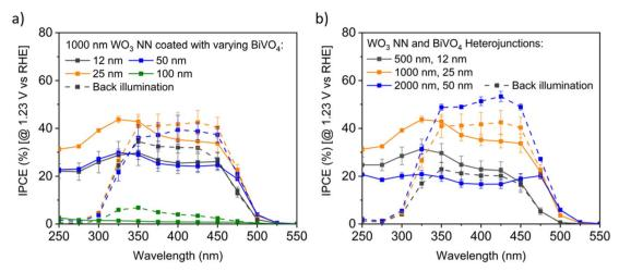
Fig. 8 Exemplar IPCE profiles for BiVO<sub>4</sub>-coated WO<sub>3</sub> on FTO, measured at pH 7 in 0.1 M KH<sub>2</sub>PO<sub>4</sub>/K<sub>2</sub>HPO<sub>4</sub> (ag.) buffer electrolyte under front and back illumination (dashed lines), with 95% confidence intervals for triplicate measurements (a) varying  $BiVO_4$  on 1000 nm long  $WO_3$  nanoneedles, and (b) constant ratio of varying BiVO<sub>4</sub> and WO<sub>3</sub> nanoneedle thicknesses
