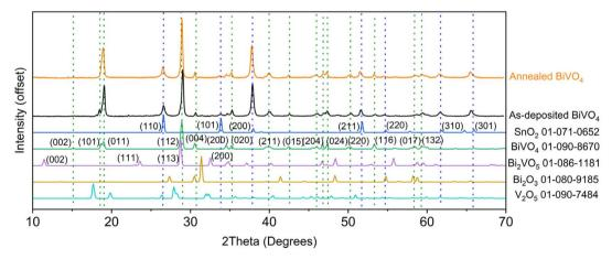
Fig. 3 XRD patterns for BiVO<sub>4</sub> films grown on FTO-coated glass by AACVD before annealing (as deposited) and after annealing at 500 °C for 2 hours in air. Data is plot alongside PDF card references patterns for SnO<sub>2</sub> (*i.e.* the FTO substrate), BiVO<sub>4</sub>, Bi<sub>2</sub>VO<sub>5</sub>, Bi<sub>2</sub>O<sub>3</sub> and V<sub>2</sub>O<sub>5</sub>.
