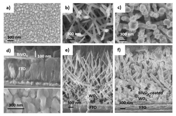
Fig. 1 Exemplar SEM images of (a) FTO substrate, (b) top view of WO<sub> $\frac{1}{3}$ </sub> NN, (c) top view of WO<sub> $\frac{1}{3}$ </sub> NN coated with 100 nm thick BiVO<sub>4</sub>, (d) (top): sideon view of 100 nm thick BiVO<sub>4</sub> on FTO, (bottom): top-down view of BiVO<sub>4</sub>, (e) side-on view of 4000 nm long WO<sub>3</sub> NN on FTO and (f) side-on view of 100 nm thick BiVO<sub>4</sub> coated on 4000 nm long WO<sub>3</sub> NN on FTO.
