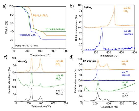
Fig. 2 TGA-mass spectrometry (MS) of the precursors used in the AACVD synthesis of BiVO<sub>4</sub> (a) weight loss % as a function of temperature, and mass spectrometry of volatile materials for (b) Bi(Ph)<sub>3</sub>, (c) V(acac)<sub>3</sub>, and (d) 1:1 mixture of Bi(Ph)<sub>3</sub> and V(acac)<sub>3</sub>.
