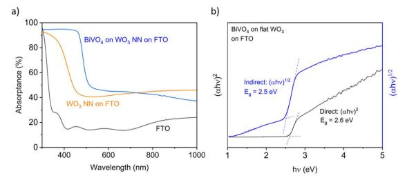
Fig. 5 (a) UV-vis absorptance for 2000 nm thick  $WO_3$  NN and 100 nm  $BiVO_4$ -coated NN  $WO_3$  compared to FTO-coated glass and (b) Tauc plots derived from measurements of transmittance and total reflectance of 400 nm planar  $BiVO_4$  on 100 nm planar  $WO_3$  on FTO-coated glass.
