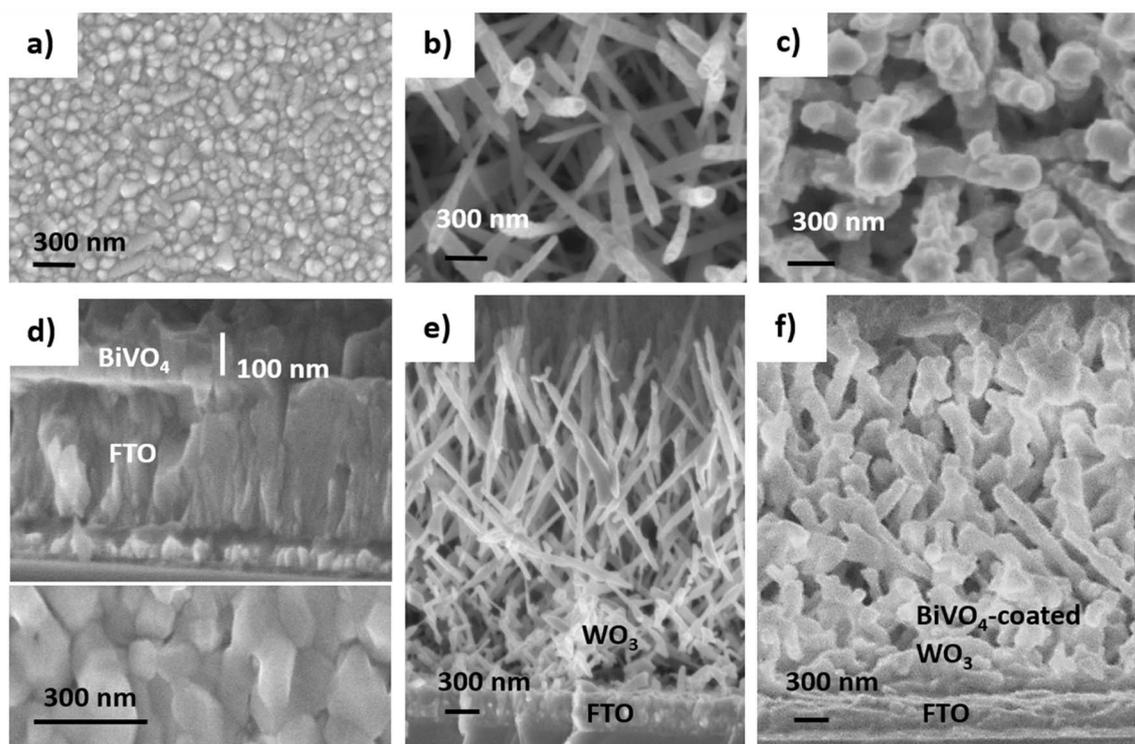
Fig. 1 Exemplar SEM images of (a) FTO substrate, (b) top view of  $\text{WO}_3$  NN, (c) top view of  $\text{WO}_3$  NN coated with 100 nm thick  $\text{BiVO}_4$ , (d) (top): side-on view of 100 nm thick  $\text{BiVO}_4$  on FTO, (bottom): top-down view of  $\text{BiVO}_4$ , (e) side-on view of 4000 nm long  $\text{WO}_3$  NN on FTO and (f) side-on view of 100 nm thick  $\text{BiVO}_4$  coated on 4000 nm long  $\text{WO}_3$  NN on FTO.
