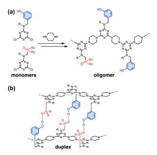
Fig. 1 (a) Recognition-encoded melamine oligomers (REMO) are synthesised from dichlorotriazine monomers using S<sub>N</sub>Ar reactions with piperazine. (b) Phenol phosphine oxide H-bonding interactions lead to the assembly of duplexes between sequence-complementary strands. R = isobutyl or 2-ethylhexyl.
