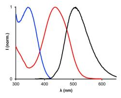
Fig. 5 Normalised UV/vis absorption spectra of 50  $\mu$ M pDDDDDDDDDDDDf (blue line) and 50  $\mu$ M pD\*AAAAAAAAAAAAA( (red line), and the fluorescence emission spectrum ( $\lambda_{ex}=348$  nm) of 0.5  $\mu$ M pDDDDDDDDDDDDDDDDf (black line). All spectra were recorded in chloroform at 298 K.
