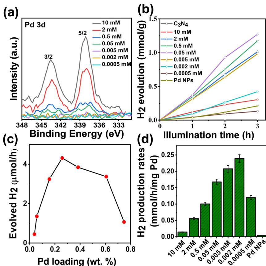
Fig. 3 (a) Pd 3d XPS spectra of Pd SAs/C<sub>3</sub>N<sub>4</sub> at different concentrations of tetraaminepalladium chloride, (b) photocatalytic H<sub>2</sub> evolution, (c) evolved H<sub>2</sub> at different Pd SA loadings, and (d) normalized H<sub>2</sub> evolution rates for different concentrations Pd SAs using tetraaminepalladium chloride.
