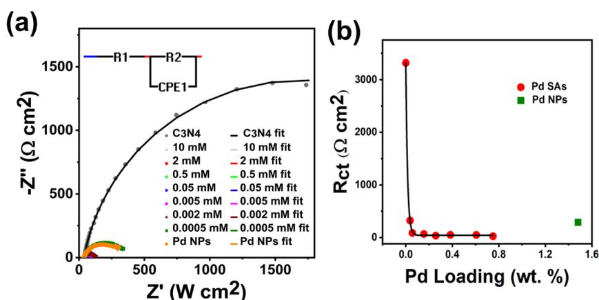
Fig. 4 (a) EIS plots of C<sub>3</sub>N<sub>4</sub>, Pd SAs/C<sub>3</sub>N<sub>4</sub> and Pd NPs/C<sub>3</sub>N<sub>4</sub> at the voltage of -0.5 V (vs. Ag/AgCl) in 0.1 M Na<sub>2</sub>SO<sub>4</sub> aqueous electrolyte. The equivalent circuit model used for fitting is depicted in the inset of (a). (b)  $R_{ct}$  vs. Pd loading plot of Pd SAs/C<sub>3</sub>N<sub>4</sub> samples.
