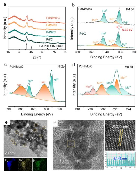
Fig. 1 (a) XRD spectra of different Pd-based catalysts; XPS spectra of (b) Pd 3d, (c) Ni 2p and (d) Mo 3d in PdNiMo/C; (e and f) TEM image and the corresponding elemental mapping images of PdNiMo/C catalysts.
