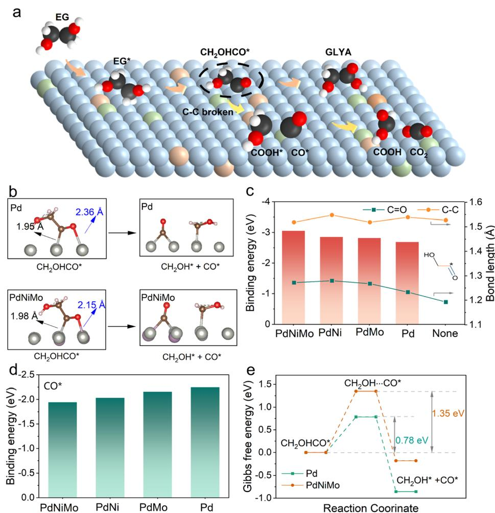
Fig. 5 (a) Reaction pathways for C–C bond breaking in the EGOR process. (b) Calculated configuration of CH<sub>2</sub>OH-CO\* and its C–C bond breaking products. Calculated adsorption energies of (c) CH<sub>2</sub>OH-CO\* and (d) CO on Pd-based electrocatalyst surfaces. (e) Calculated Gibbs free energy change during C–C bond cleavage in CH<sub>2</sub>OH-CO\* on Pd and PdNiMo surfaces.
