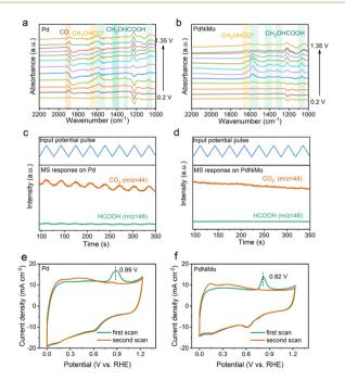
Fig. 4 Electrochemical in situ FTIR spectra of (a) PdNiMo/C and (b) Pd/C in 1.0 M KOH + 1.0 M EG. The in situ mass spectra of (c) PdNiMo/C and (d) Pd/C. CO stripping of (e) PdNiMo/C and (f) Pd/C with a scan rate of 5 mV s $^{-1}$ .
