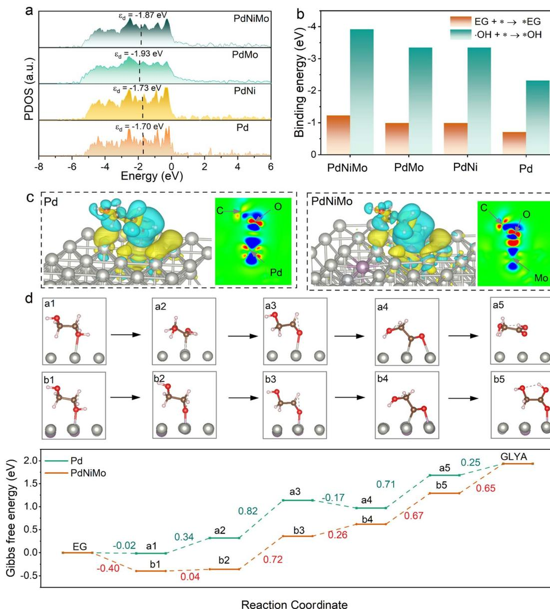
Fig. 3 (a) PDOS (d-band) of PdNiMo, PdMo, PdNi, and Pd. (b) Calculated adsorption energies of EG and \*OH. (c) Charge density difference during EG adsorption onto PdNiMo and Pd (111); negative and positive charges are presented in green and yellow, respectively. (d) Gibbs free energy diagram and the optimized configurations of EG oxidation to GLYA on Pd and PdNiMo. The colored values are the Gibbs free energy changes in eV.
