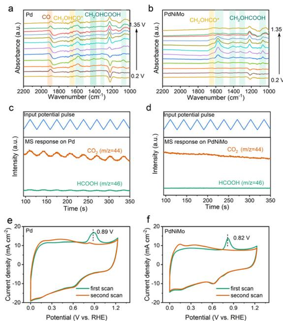
Fig. 4 Electrochemical *in situ* FTIR spectra of (a) PdNiMo/C and (b) Pd/C in 1.0 M KOH + 1.0 M EG. The *in situ* mass spectra of (c) PdNiMo/C and (d) Pd/C. CO stripping of (e) PdNiMo/C and (f) Pd/C with a scan rate of  $5$   $mV s^{-1}$ .
