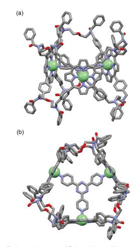
Fig. 3 Single crystal structure of **6b** from side view (a) and top view (b). The solvents, counterions and H atoms have been omitted for clarity. Color code: gray = C; red = O; blue = N; green =  $Zn^{2+}$ .
