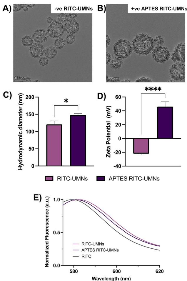
Fig. 3 Representative transmission electron micrographs of (A) RITC-UMNs and (B) APTES RITC-UMNs. (C) Hydrodynamic diameter and (D)  $\zeta$ -potential of RITC-UMNs and APTES RITC-UMNs. Error bars represent the standard deviation of 3 material replicates. (E) Fluorescence emission spectra of RITC-UMNs, APTES RITC-UMNs, and RITC alone. Unpaired *t*-tests were used to evaluate statistical significance ( $*p < 0.05$ ,  $****p < 0.0001$ ).
