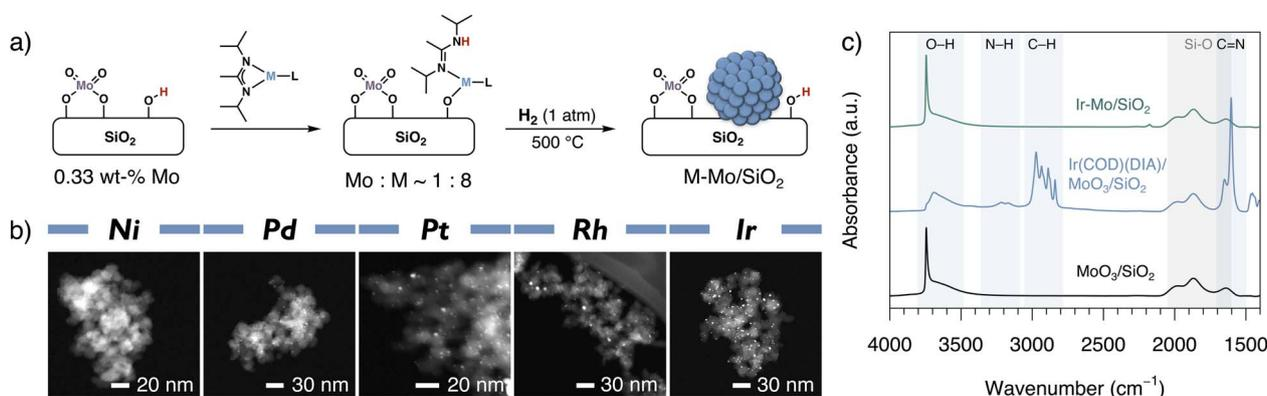
Fig. 1 (a) General synthesis route of bimetallic materials. (b) HAADF-STEM micrographs of bimetallic M–Mo/SiO<sub>2</sub> materials. (c) IR spectra of MoO<sub>3</sub>/SiO<sub>2</sub> (black spectrum), Ir(COD)(DIA)/MoO<sub>3</sub>/SiO<sub>2</sub> (blue spectrum), Ir–Mo/SiO<sub>2</sub> (green spectrum).
