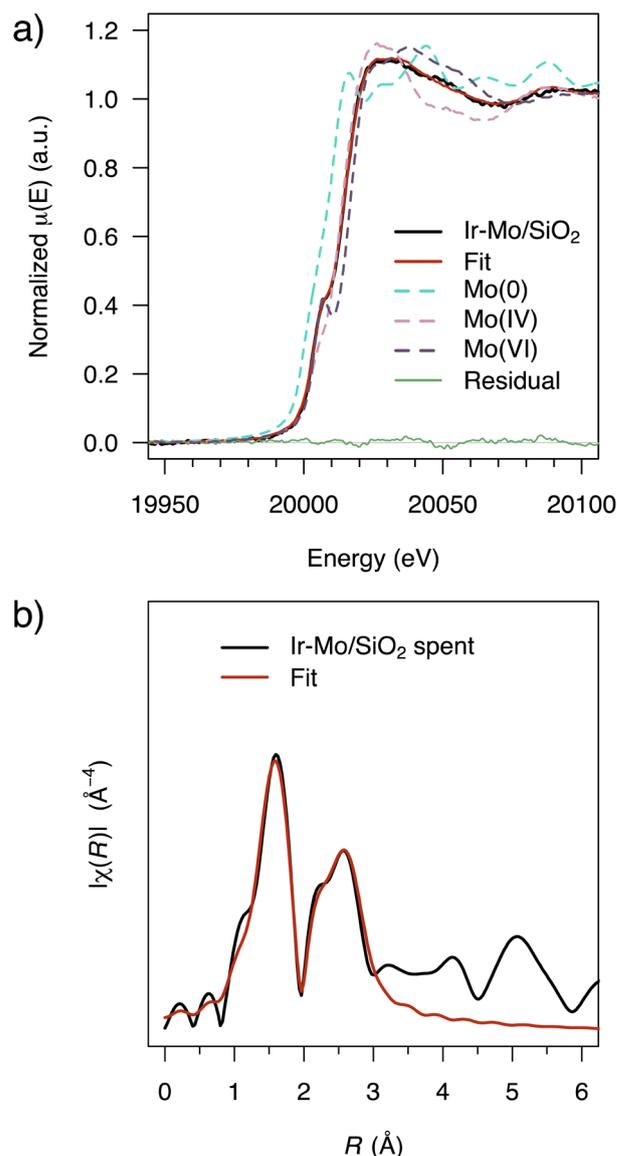
Fig. 4 (a) LCF of fresh Ir–Mo/SiO<sub>2</sub> with Mo(vi), Mo(IV), and Mo(0) references of Mo K-edge XANES spectra. (b) Mo K-edge EXAFS spectrum and fit of spent Ir–Mo/SiO<sub>2</sub> after HDO of 1-nonanol.
