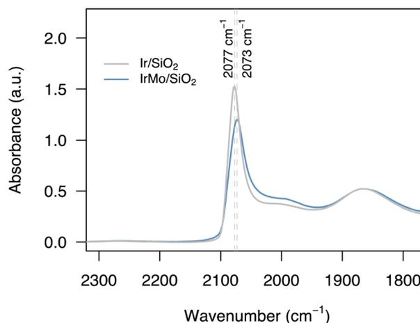
Fig. 3 IR spectra of adsorbed CO on Ir/SiO<sub>2</sub> (grey spectrum) and Ir–Mo/SiO<sub>2</sub> (blue spectrum) after dosing *ca.* 15 mbar of CO, followed by evacuation at 10<sup>-5</sup> mbar for 10 minutes. The spectra are baseline corrected and normalized by the intensity of the siloxane band at 1870 cm<sup>-1</sup>.
