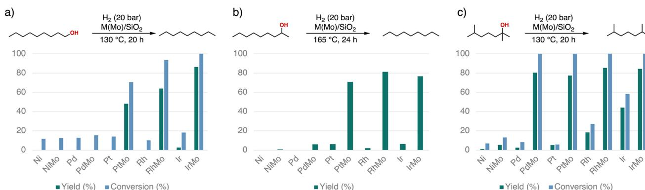
**Fig. 2** Conversion and HDO product yields for mono- and bimetallic materials in the deoxygenation of (a) 1-nonanol, (b) 2-nonanol, and (c) 2,6-dimethylheptan-2-ol. Solvent = decahydronaphthalene (decalin). The conversion of 2-nonanol could not be determined due to the overlap of the 2-nonanol GC signal with one isomer of decalin.
