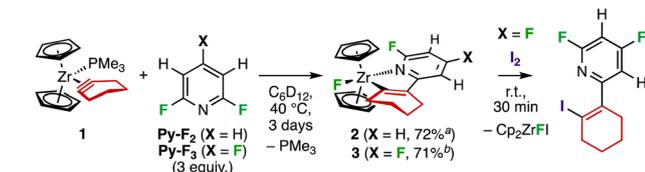
Scheme 2 Reaction of **1** with Py-F<sub>n</sub> (n = 2, 3) leads to C–F alkenylation. <sup>a</sup>NMR yield. <sup>b</sup>Isolated yield.
