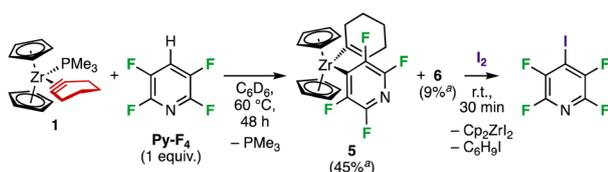
Scheme 3 Reaction of **1** with **Py-F<sub>4</sub>** leads to C–H activation. <sup>a</sup>NMR yields.
