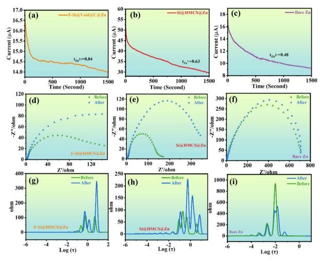
Fig. 3 (a-c) Current-time plot of assembled symmetric cells of bare Zn, Si@HMCS@Zn, and F-Si@HMCSC@Zn after constant potential polarization at 15 mV. (d-i) EIS curves and DRT analysis before and after polarization for (d and g) F-Si@HMCS@Zn, (e and h) Si@HMCS@Zn, and (f and i) bare Zn.
