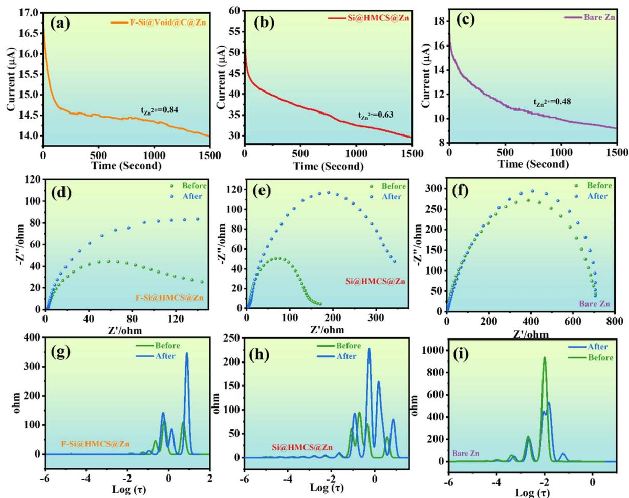
Fig. 3 (a–c) Current-time plot of assembled symmetric cells of bare Zn, Si@HMCS@Zn, and F-Si@HMCS@Zn after constant potential polarization at 15 mV. (d–i) EIS curves and DRT analysis before and after polarization for (d and g) F-Si@HMCS@Zn, (e and h) Si@HMCS@Zn, and (f and i) bare Zn.
