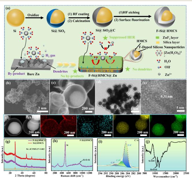
Fig. 1 (a) The synthesis process of F-Si@HMCS and schematic illustrations of Zn metal plating behaviors on bare Zn and F-Si@HMCS@Zn electrodes. (b and c) SEM images; (d) TEM image; (e) HRTEM image; (f) the corresponding energy-dispersive X-ray mapping of F-Si@HMCS. (q) XRD pattern; (h) Raman spectrum of F-Si@HMCS. XPS spectrum of F-Si@HMCS: (i) C 1s. (j) FTIR spectrum of F-Si@HMCS.
