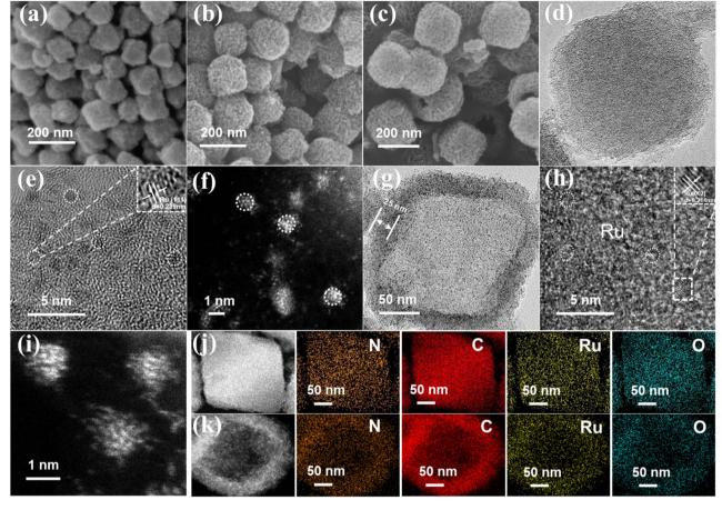
Fig. 1 SEM image of UiO-66-NH<sub>2</sub> (a), c-Ru@NPC (b) and c-Ru@H-NPC (c). (d) (g) TEM image of c-Ru@NPC and c-Ru@H-NPC. (e) (h) Highresolution TEM image of c-Ru@NPC and c-Ru@H-NPC. (f) (i) ac-STEM image of c-Ru@NPC and c-Ru@H-NPC. (j) (k) HAADF-STEM image and corresponding EDS mapping images of N, C, Ru and O of c-Ru@NPC and c-Ru@H-NPC.
