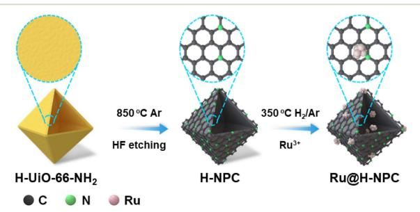
Scheme 1 Synthesis of a hollow c-Ru@H-NPC catalyst.
