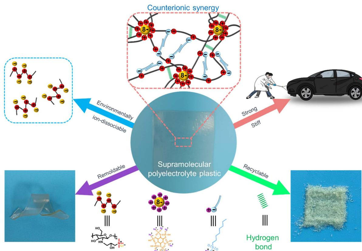
**Scheme 1** Schematic diagram of the fabrication of environmentally ion-dissociable high-performance supramolecular polyelectrolyte plastics with a synergistic multivalent and hydrophobic counterion strategy.
