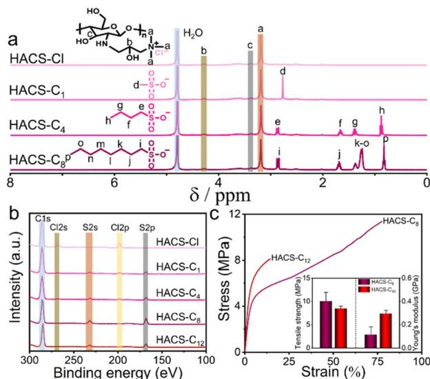
Fig. 1 Characterization of cationic polyelectrolytes HACSs with different monovalent counterions. (a)  $^1\text{H}$  NMR spectra and (b) XPS analyses of HACS-Cl and HACS- $\text{C}_x$  materials. (c) Representative stress–strain curves for HACS- $\text{C}_8$  and HACS- $\text{C}_{12}$  with the inset showing the tensile strengths and Young's moduli.
