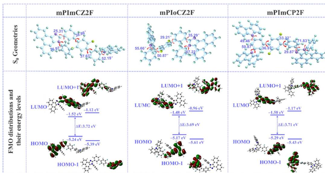
Fig. 2 Molecular geometries in the ground state, FMO distributions and calculated energy levels of mPImCZ2F, mPloCZ2F and mPImCP2F.
